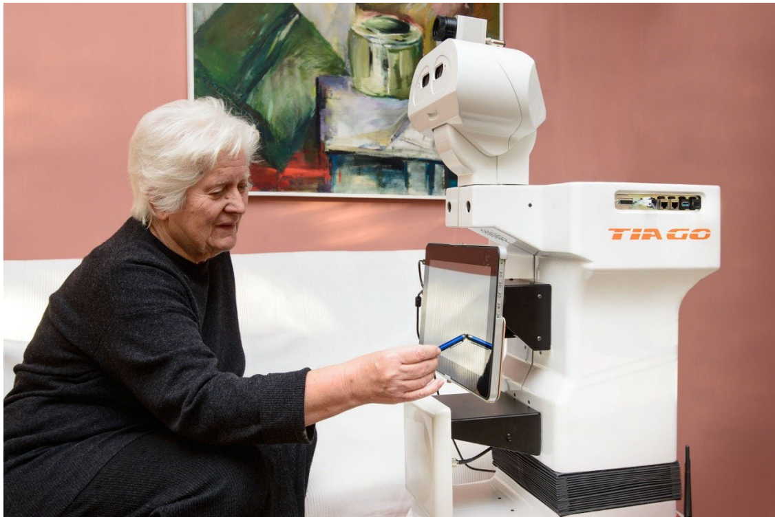
Figure 2.89: The Tiago platform interacting with an older individual through the touch screen. Image credit: Pal Robotics.
