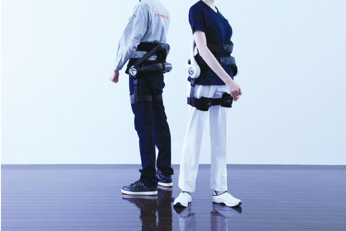
Figure 3.16: HAL Lumbar Type is an application designed to solve the physical burden in healthcare environment from two directions with a single unit: Supporting caregivers with heavy lifting and training the body core and lower limb functions of seniors. Image credit: Prof. Sankai, University of Tsukuba/Cyberdyne Inc.
