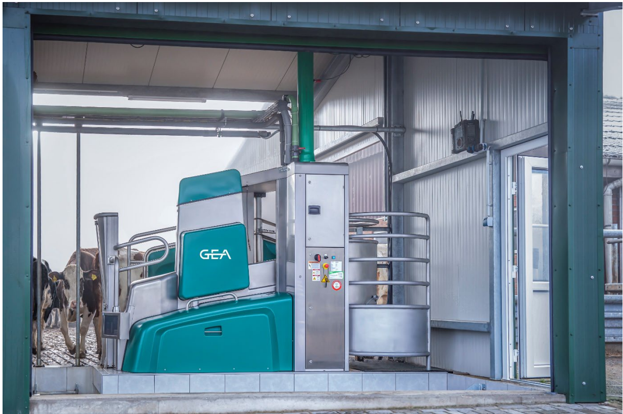
Figure 2.16: The Dairyrobot R9500 is engineered to enhance the milking process for the cow. GEA's proven In-Liner Everything technology performs every step of the milking process – stimulating, teat cleaning, fore-stripping, milk harvesting, and post-dipping – in a single attachment. This process, which occurs within the teat cup, is key to harvesting quality milk while maximizing the efficiency of a robotic milking facility. Image credit: GEA.
