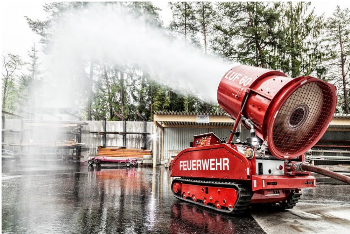
Figure 2.79: The tele-operated firefighting robot with tracked undercarriage LUF 60 is a vehicle for operations under difficult conditions, which can produce a nebulized water jet of up to 2,400 liters of water per minute. Image credit: LUF GmbH.
