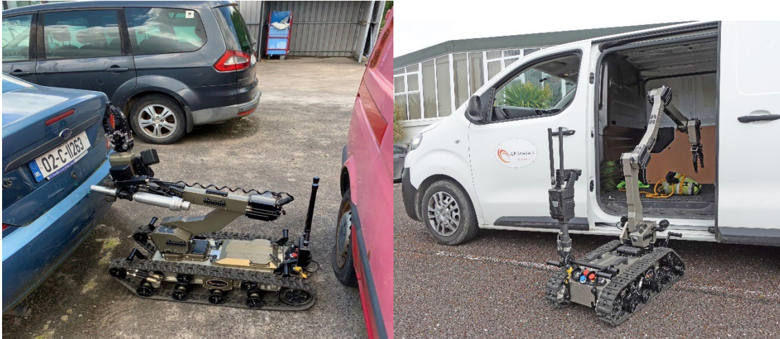
Figure 2.84: Avenger Lite is a compact mid-sized robot with the ability to access tight spaces while still deploying EOD render safe tools, equipment, and sensors common to the entire Avenger family of robots (left). Avenger 2.0 includes a manipulator arm with seven degrees of freedom, offering the necessary reach and lift for EOD operations (right). Image credit: Med-Eng.
