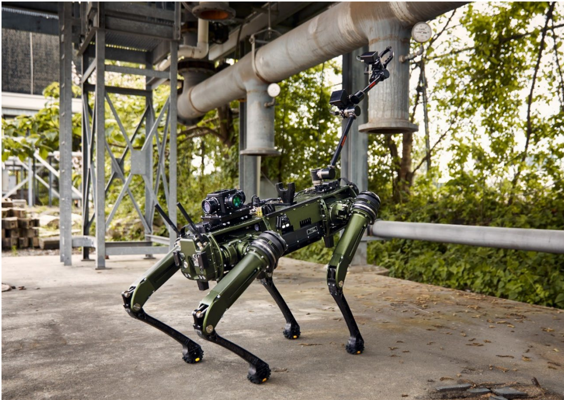
Figure 3.35: Vision 60 Quadrupedal Uncrewed Ground Vehicle is used for various industrial inspection applications. Image credit: Ghost Robotics.
