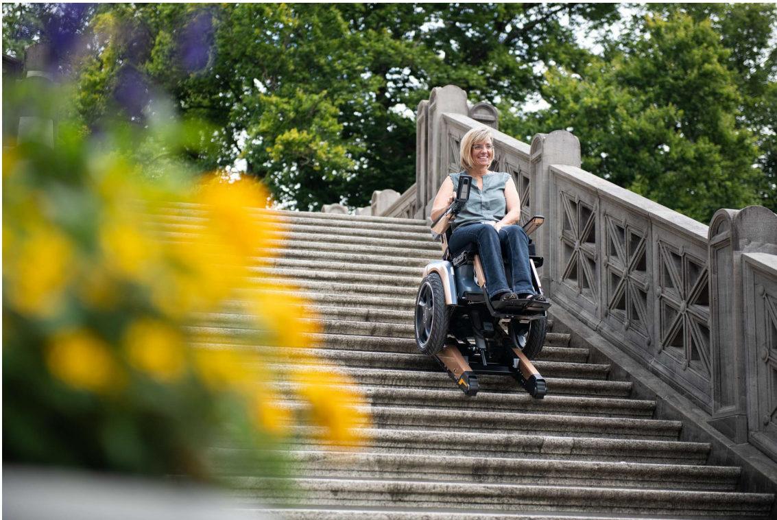
Figure 4.17: Scewo power wheelchair easily overcomes various obstacles thanks to the built-in chains. Image credit: Scewo AG.
