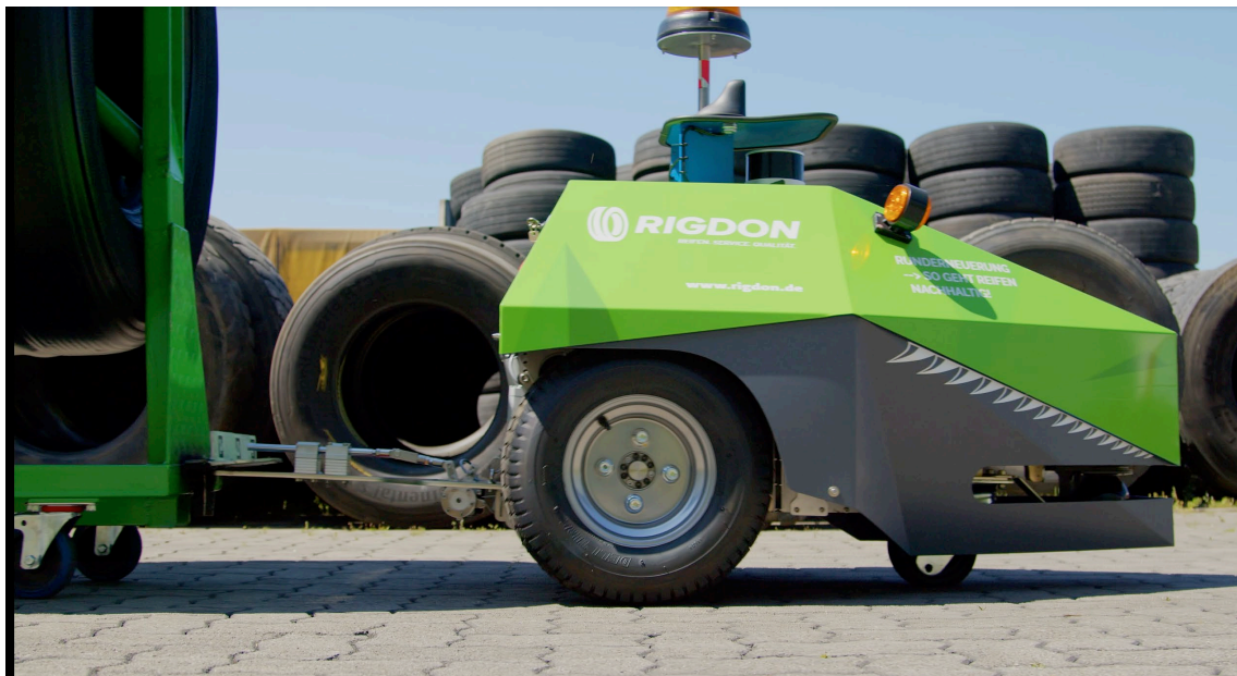
Figure 6.8: The Innok Robotics AMR Induros autonomously moves tyres from outdoor storage to the production stations at the Innok customer Rigdon. Image credit: Innok Robotics.
