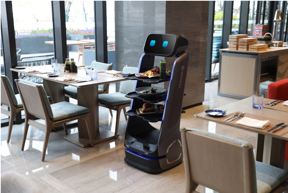
Figure 2.65: Restaurant/hotel delivery robot T9 with a payload of 40 kg or 10kg per layer from Keenon. Image credit: Keenon.
