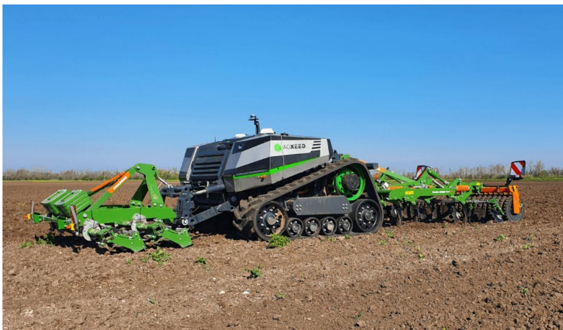
Figure 2.8: Agbot 5.115T2 with implements for soil preparation. Seedbed preparation can be performed with a speed of up to 11km/h. Image credit: Agxeed.
