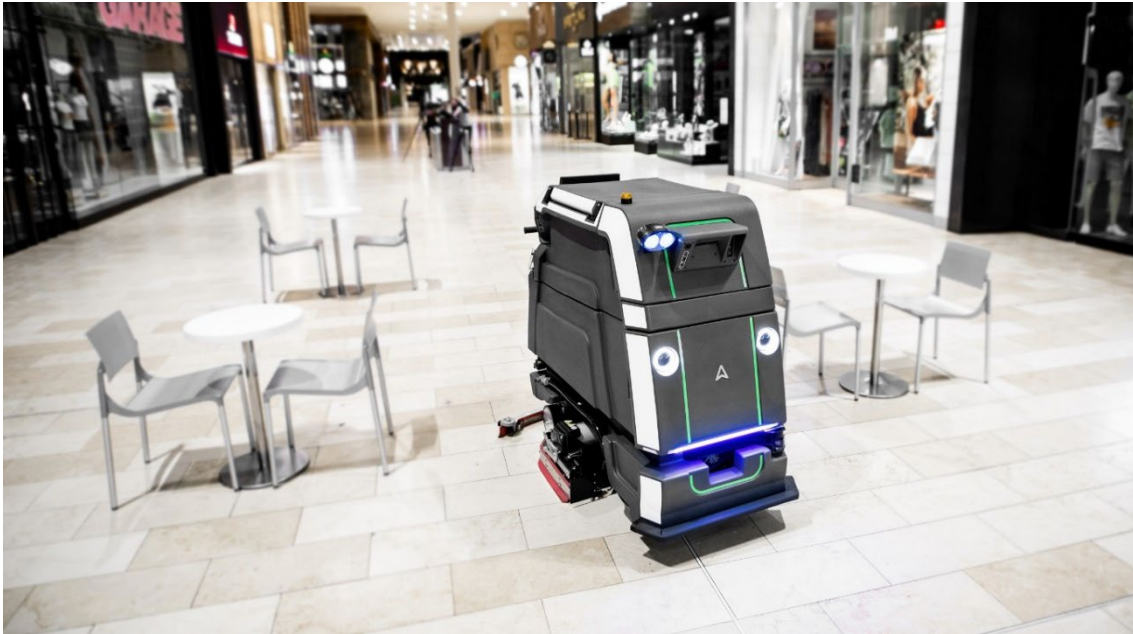
Figure 2.22: Neo 2 is a fully autonomous floor scrubbing robot chosen by organizations around the world and deployed in a variety of commercial environments, including warehouses, shopping malls, box stores, airports, train stations, schools, universities, and hospitals. Image credit: Avidbots.
