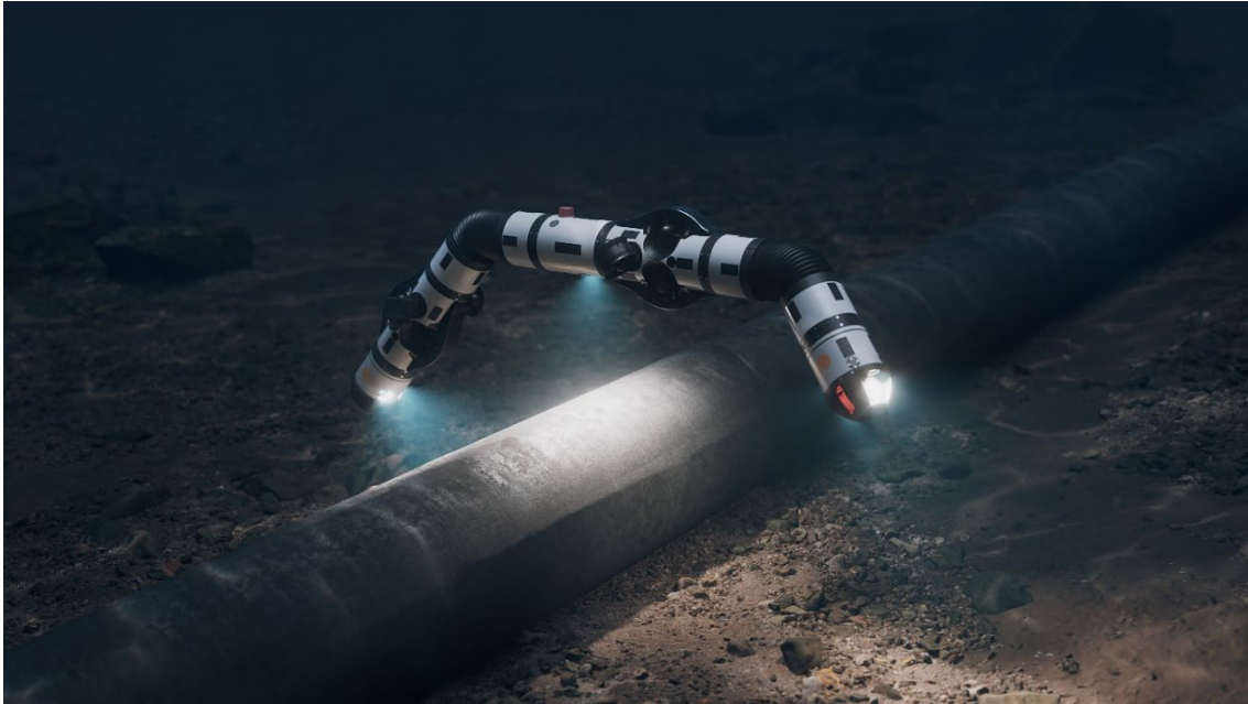
Figure 2.46: The Eelume vehicle, a self-propelled, autonomous robotic arm, inspects subsea structures. Image credit: Eelume.
