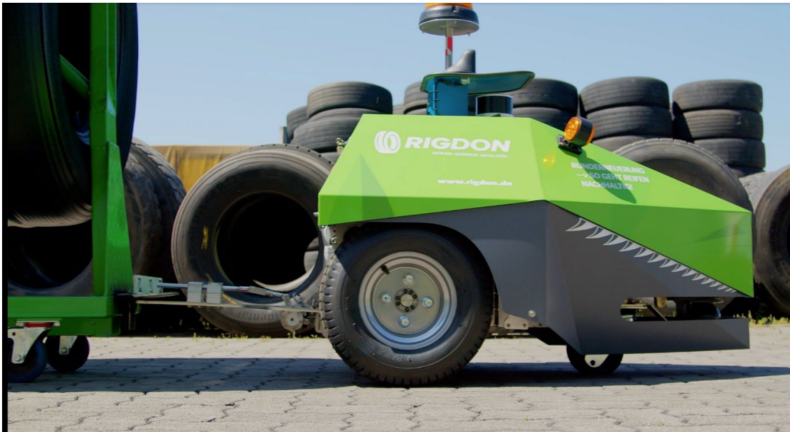
Figure 2.70: The Innok Robotics AMR Induros autonomously moves tires from the outdoor storage to the production stations at the Innok customer Rigdon. Image credit: Innok Robotics.
