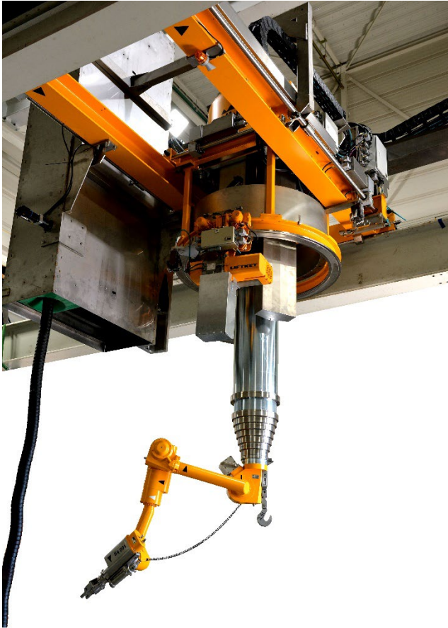
Figure 2.50: Power Manipulator equipped with a robotic arm type A1000S. Image credit: Wälischmiller Engineering GmbH.
