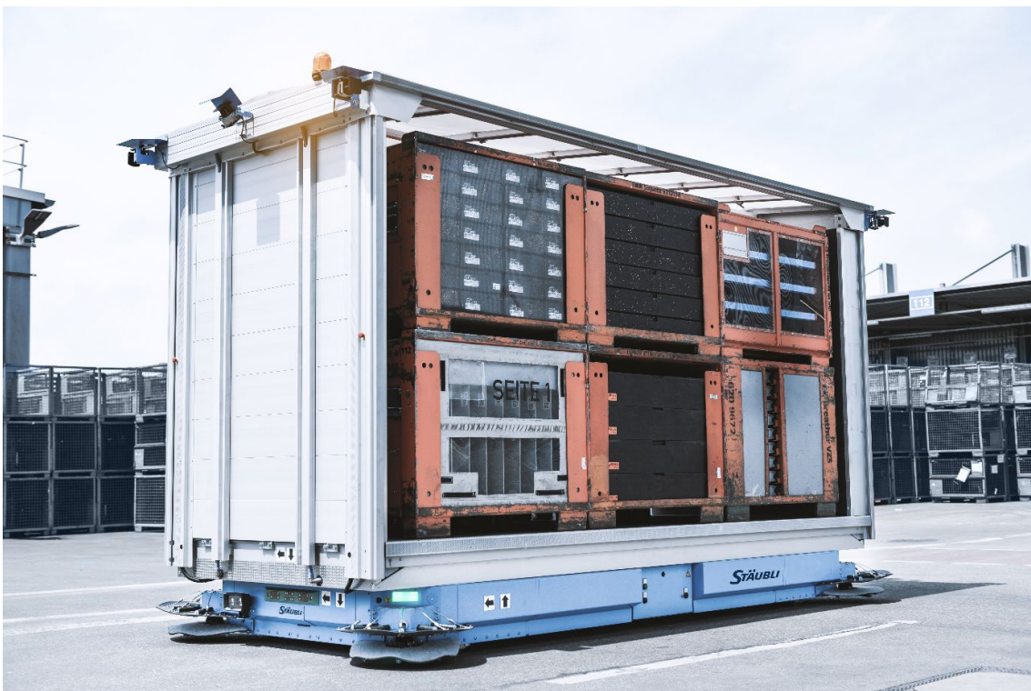
Figure 2.68: The Stäubli PF10 moves up to 10 tons and automatically connects different manufacturing halls in the automotive industry. Image credit: Stäubli.
