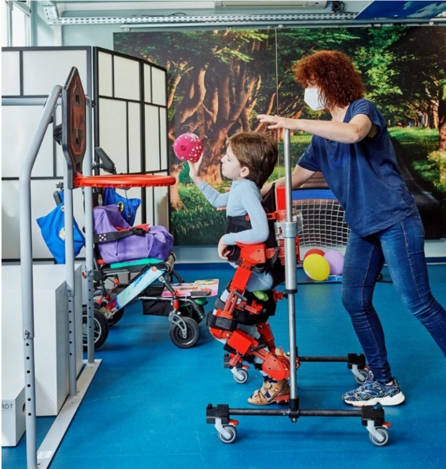
Figure 3.5: Atlas 2030 pediatric gait exoskeleton from Marsi Bionics improves the quality of life of children affected by neurological diseases. Image credit: Marsi Bionics.
