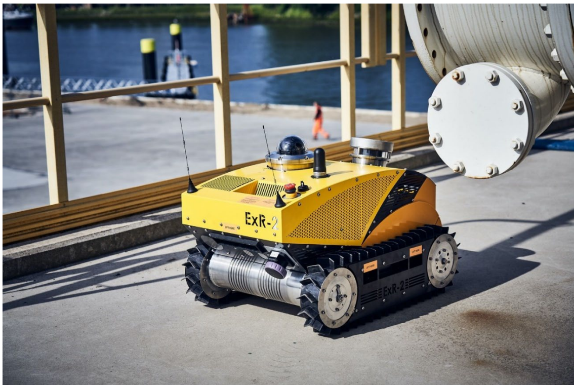
Figure 2.36: The ExR-2 is designed to support operations fully autonomously when investigating potential hazardous situations, with a light detection and range (LiDAR) and AI/ML computer on board that enable the robot to autonomously navigate in a complex environment. Image credit: Exrobotics.
