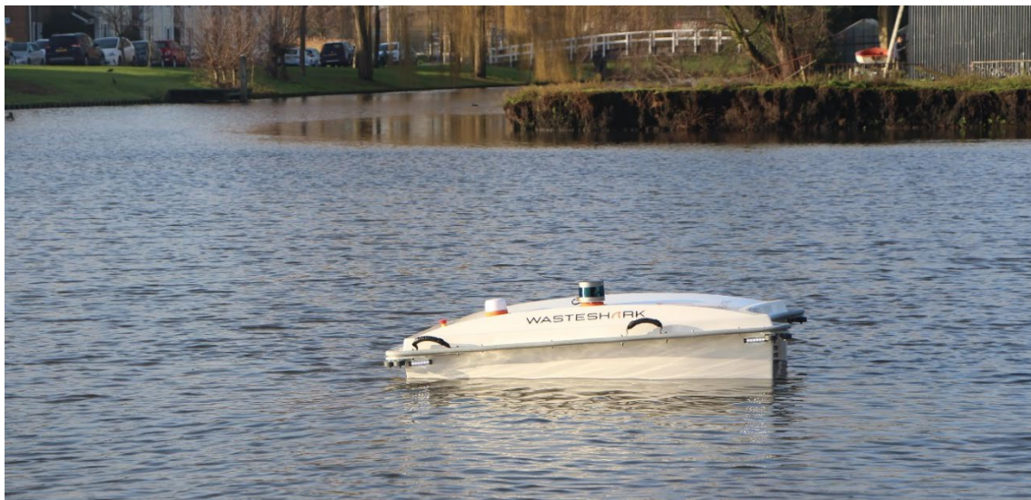
Figure 2.34: Ranmarine Technology specializes in the design and development of industrial autonomous surface vessels (ASVs) for ports, harbors, and other marine and water environments. Ranmarine's current products include the Wasteshark™ range, designed and used to clear plastics, bio-waste, and other debris from waterways. The data enablement of the products allows customers to closely monitor the environment and makeup of their water. This creates an accurate picture of the water's DNA to pinpoint any unquantified concerns. Ranmarine products are designed to be used manually or autonomously with online control and access. Image credit: Ranmarine Technology.
