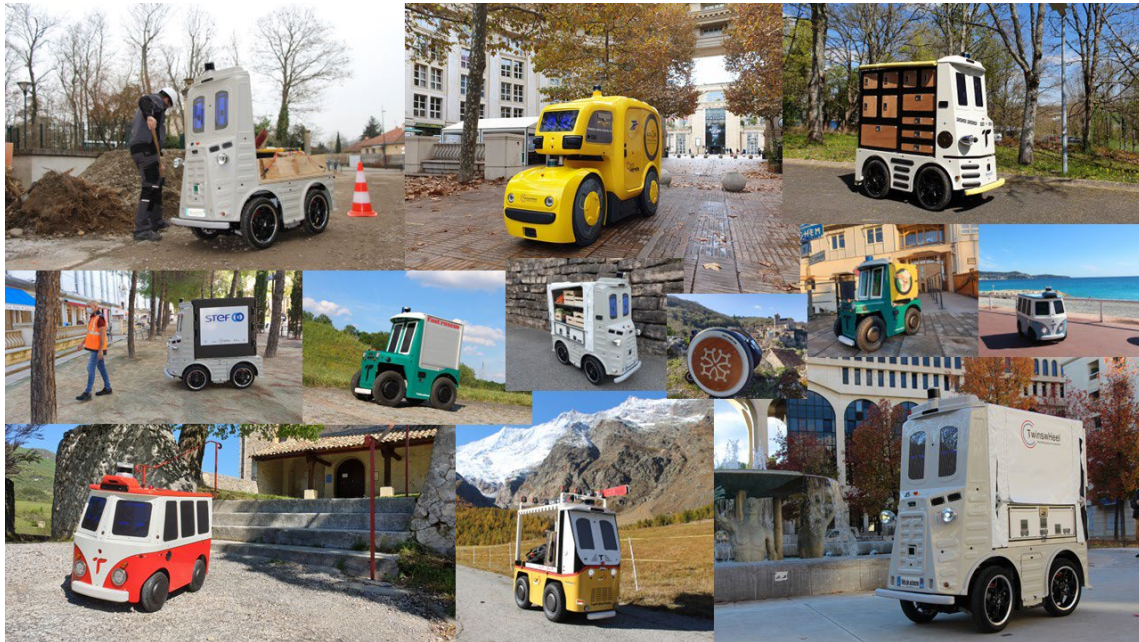
Figure 2.72: The TwinswHeel droids are autonomous mobile robots for urban logistics. ciTHy S, ciTHy M, and ciTHy L can carry 50 kg, 150 kg, and 300 kg respectively. The droids are in operation in France, Switzerland, and Germany. Image credit: Twinswheel.
