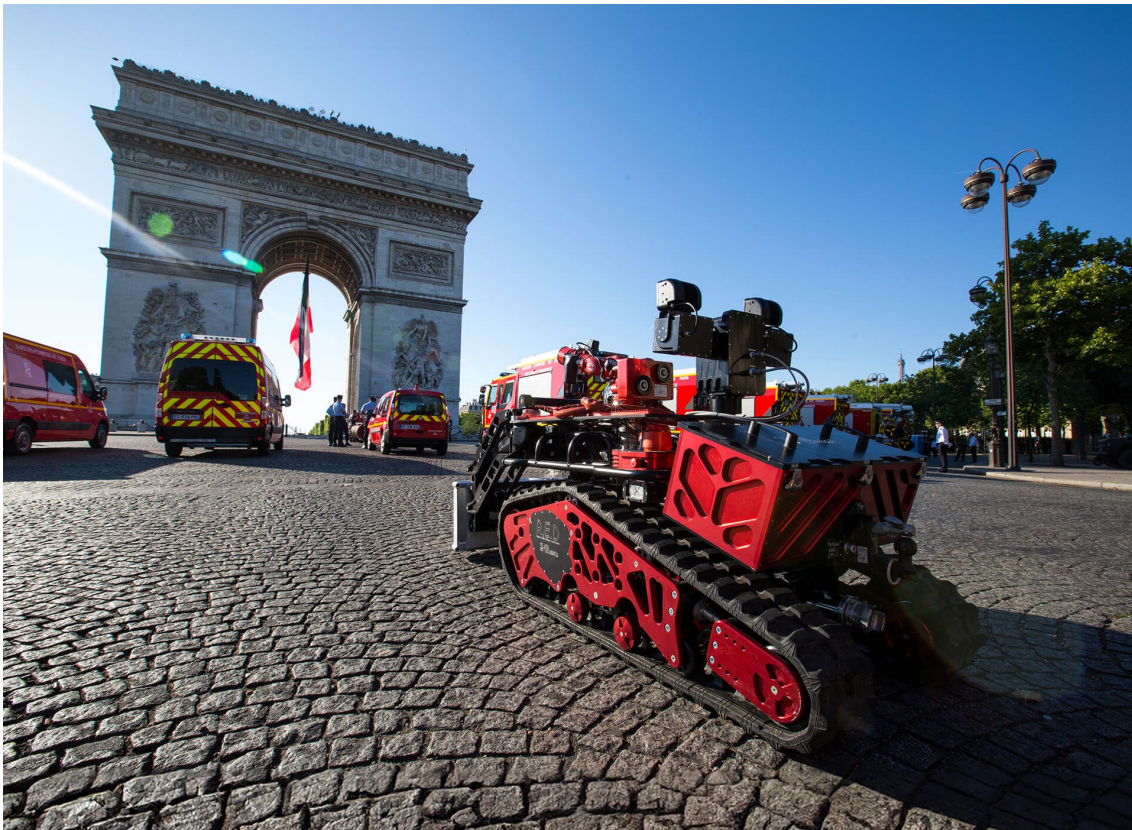
Figure 2.80: Shark Robotics offers the Colossus uncrewed system for extinguishing fires, transporting equipment or casualties, providing relevant information thanks to gas and temperature sensors, and enabling day/night and thermal vision to locate people even in smoke. Image credit: Shark Robotics.
