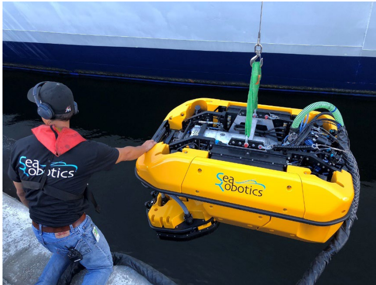
Figure 2.26: The Hullbug, Hull Bio-inspired Underwater Grooming system, is a modular system that can be operated remotely or work autonomously. The interchangeable grooming/cleaning tools form the front of the system and range from light brushing tools for biofilm removal to dual cavitating water jet tools. Image credit: Searobotics.
