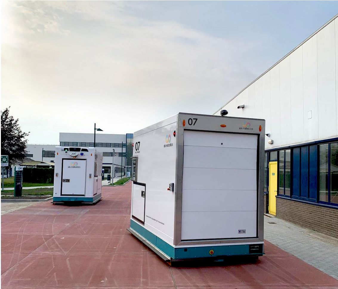
Figure 2.69: The automated guided vehicles for combined indoor and outdoor operation from Ek Robotics continuously transport goods between production halls and warehouses and are equipped with weatherproof superstructures. Image credit: Ek Robotics GmbH.
