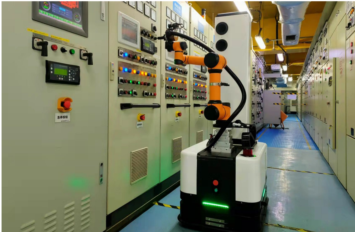
Figure 2.40: Risk of electric shock in the switchroom can be prevented by automatic inspection and operation solutions with Youibot's robot. Image credit: Shenzhen Youibot Robotics Co., Ltd.
