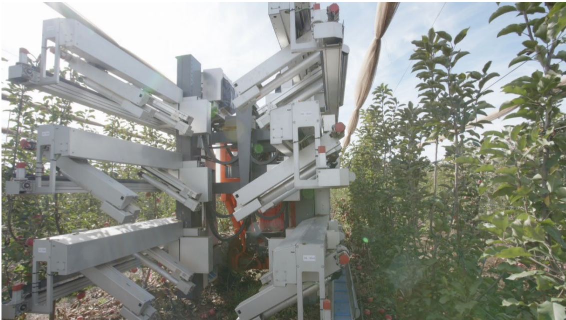
Figure 2.11: FFRobotics has introduced a robot that manages the harvesting of apples through a versatile gripper transport system. Image credit: FFRobotics.
