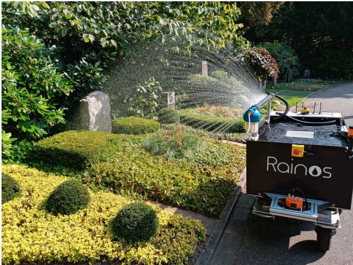
Figure 2.14: The Rainos irrigation robot from Innok Robotics autonomously waters the green areas and beds of cemeteries. By closing off the cemeteries at night, the robots can work largely undisturbed. Image credit: Innok Robotics.
