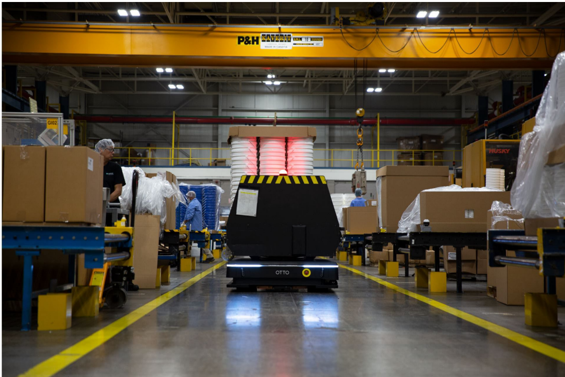
Figure 2.55: The Otto 1500 AMR delivers payloads of up to 1900 kg for Mauser Packaging. Image credit: Otto Motors.
