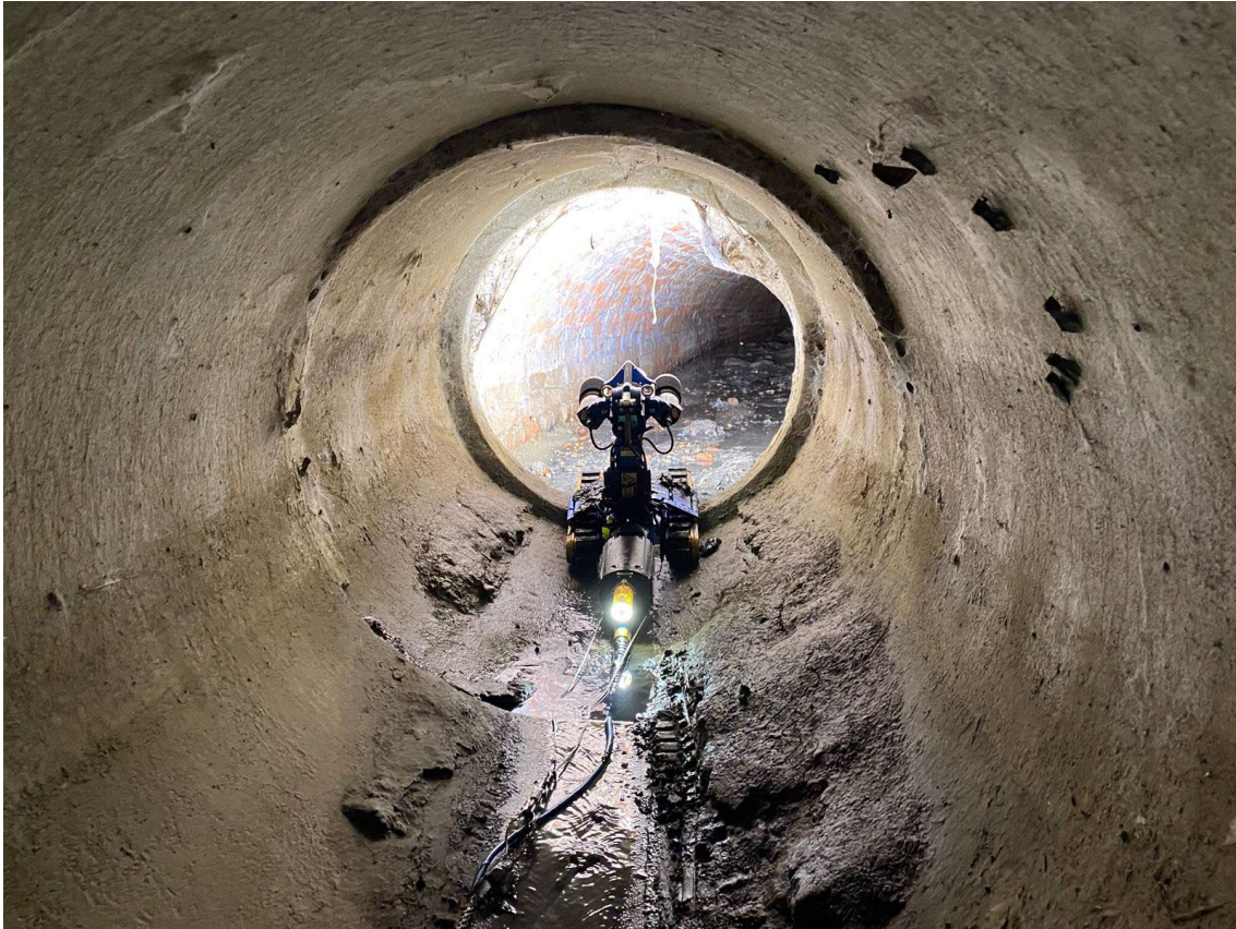
Figure 2.43: Eddyfi Technologies' Versatrax™ P-Series pipe inspection robotic crawler for long-range inspections. Image credit: Eddyfi Technologies.
