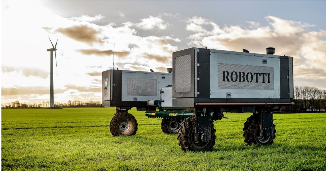
Figure 2.4: Agrobot's Robotti is an approach where the actual implement is autonomized. Many common agricultural implements can be clamped into the robotic device. Image credit: Agrobot.
