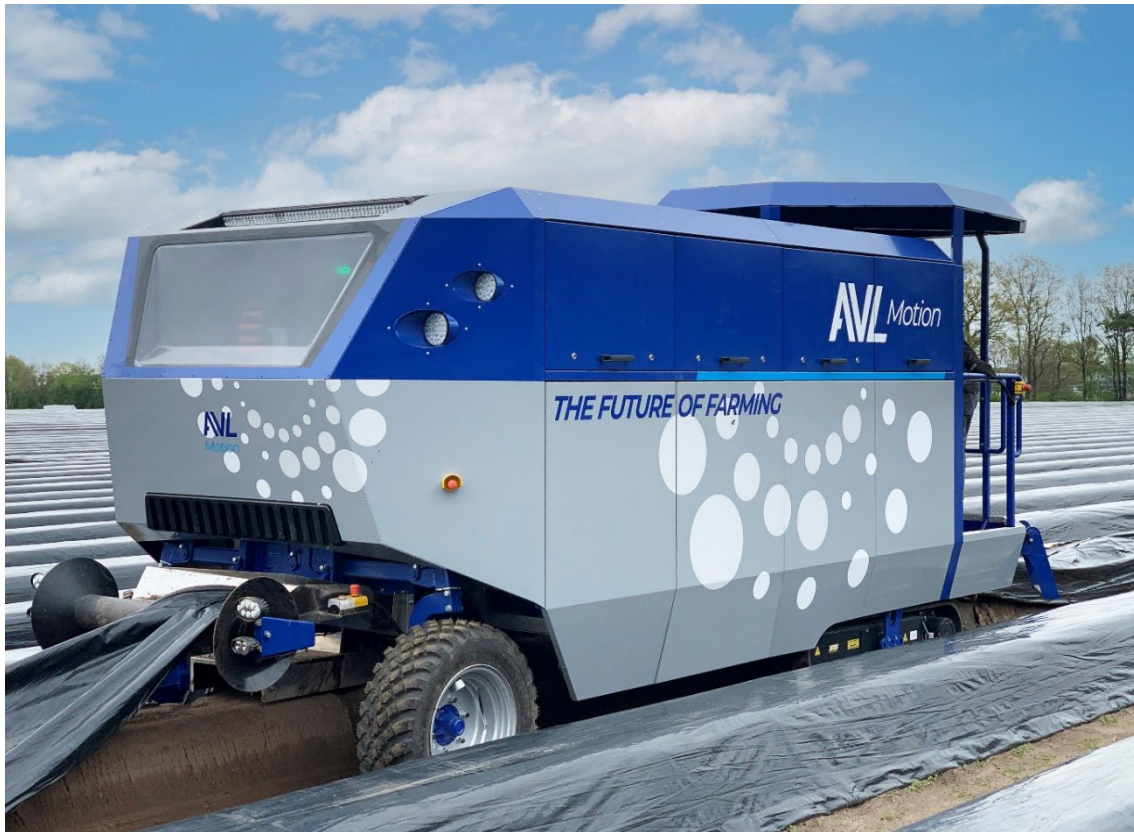
Figure 2.12: AVL's full harvesting robot for asparagus can support the scarce resource of labor in asparagus cultivation. Image credit: AVL Motion Groep B.V.
