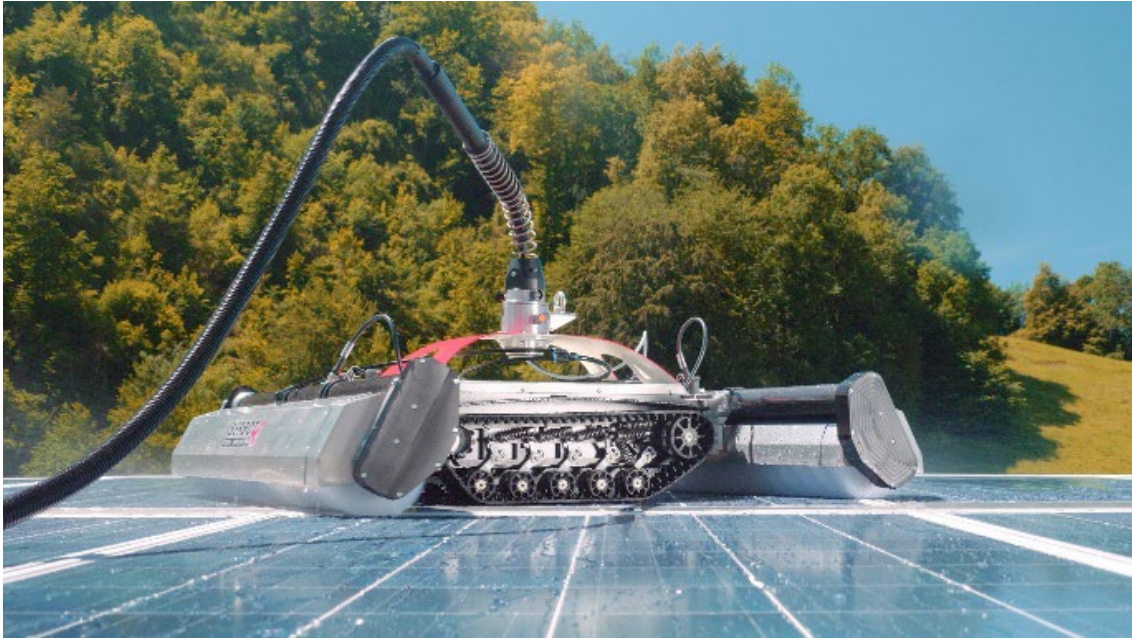
Figure 3.32: Serbot pvClean is an efficient and attractively priced solar panel/glass surface-cleaning device for inclination angles of between 15° and 20°. Image credit: Serbot.
