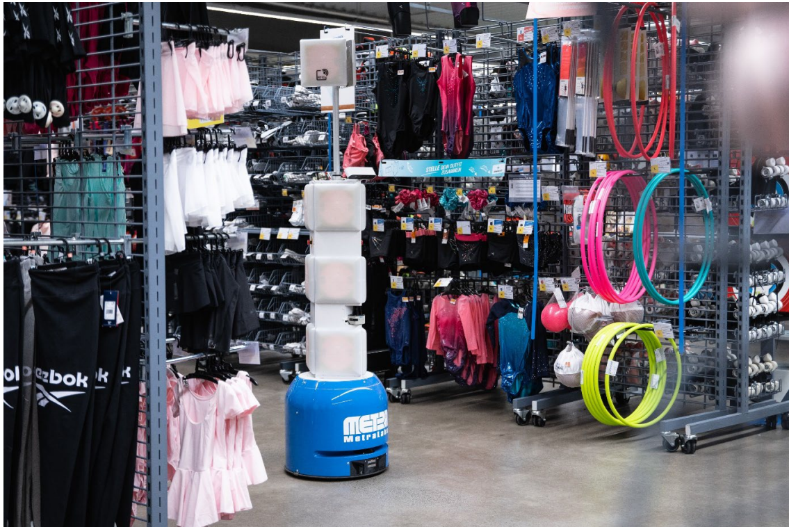
Figure 2.76: Tory RFID is an inventory robot that recognizes and captures RFID tagged articles in stores and warehouses. Image credit: Decathlon Germany.
