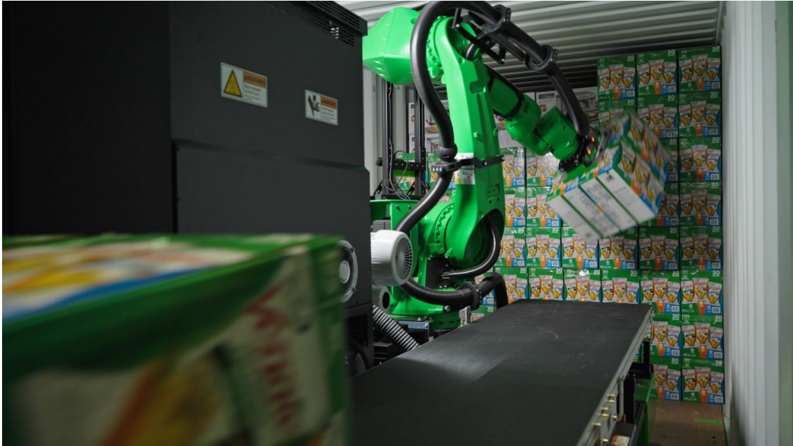
Figure 2.57: A robot from Pickle Robot unloading four food boxes. Image credit: Pickle Robot.
