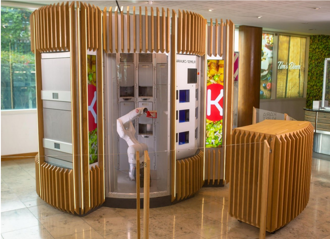
Figure 2.87: 17 ingredients, 2,700 combinations, and up to 110 meals per hour: The canteen robot Semblr tickles the tastebuds of Ocado employees with a Kuka KR Agilus. The brains behind Semblr can be found at the integrator Karakuri, a London-based startup. Image credit: Kuka Group.
