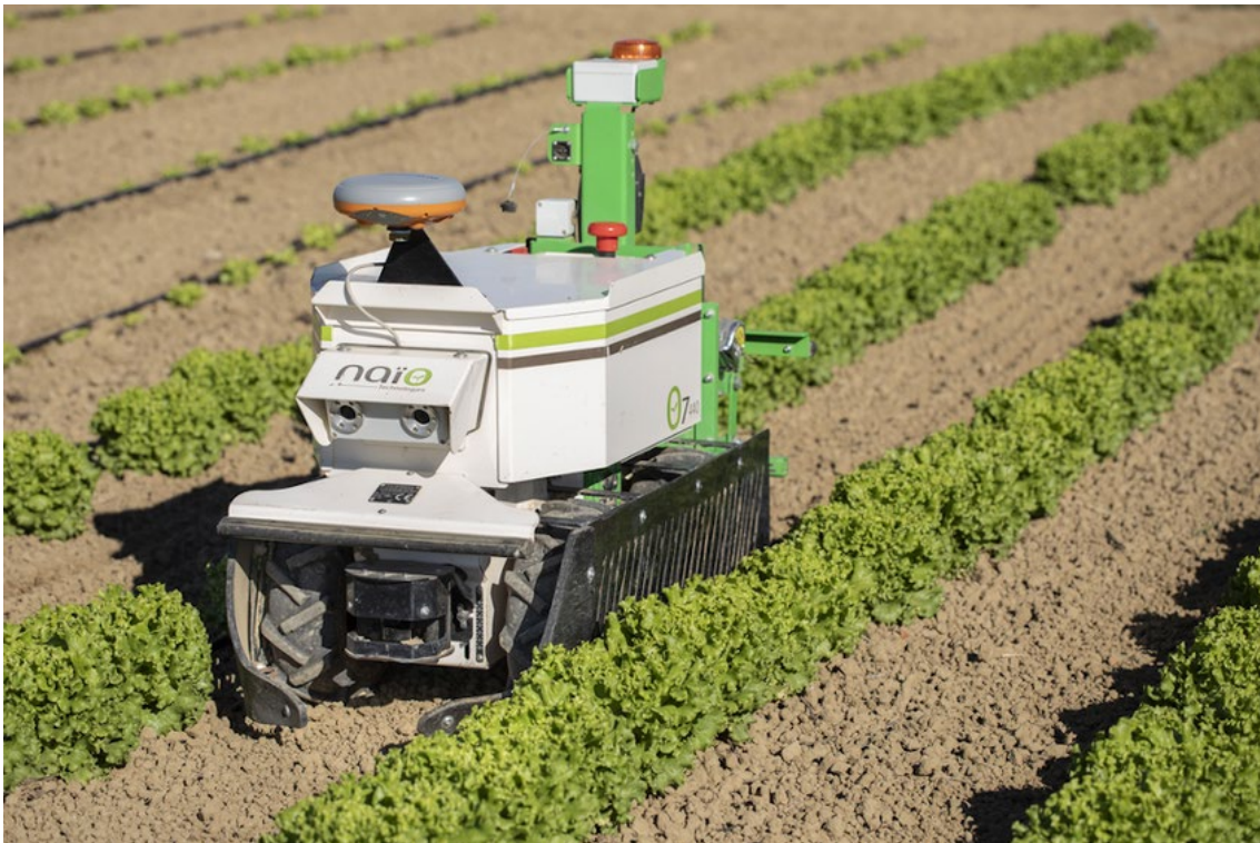
Figure 2.10: With Oz, Naïo Technologies has launched one of the smallest robots for professional weed control. Like conventional tractors, it can integrate various tools and work with them. Image credit: Naïo Technologies.
