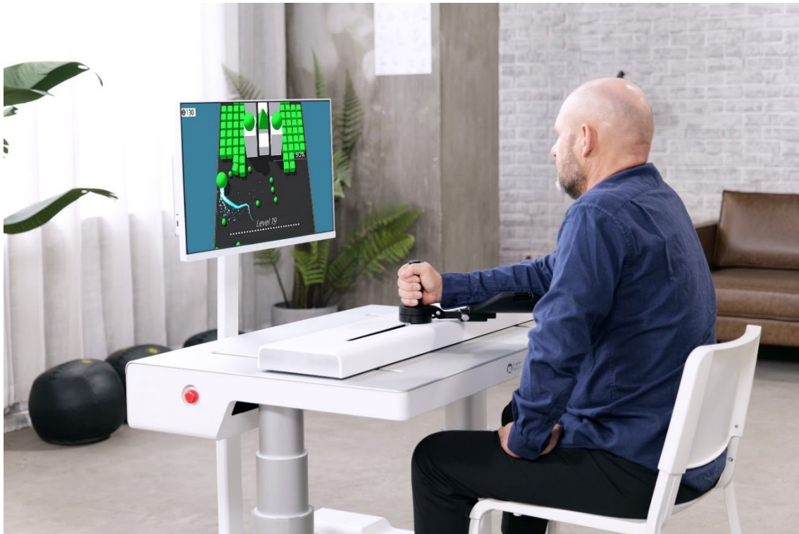
Figure 3.14: Upper limb rehabilitation robotics that simulates a mechanical environment for the users through the force feedback algorithm and high-performance motor. Image credit: Fourier Intelligence International.
