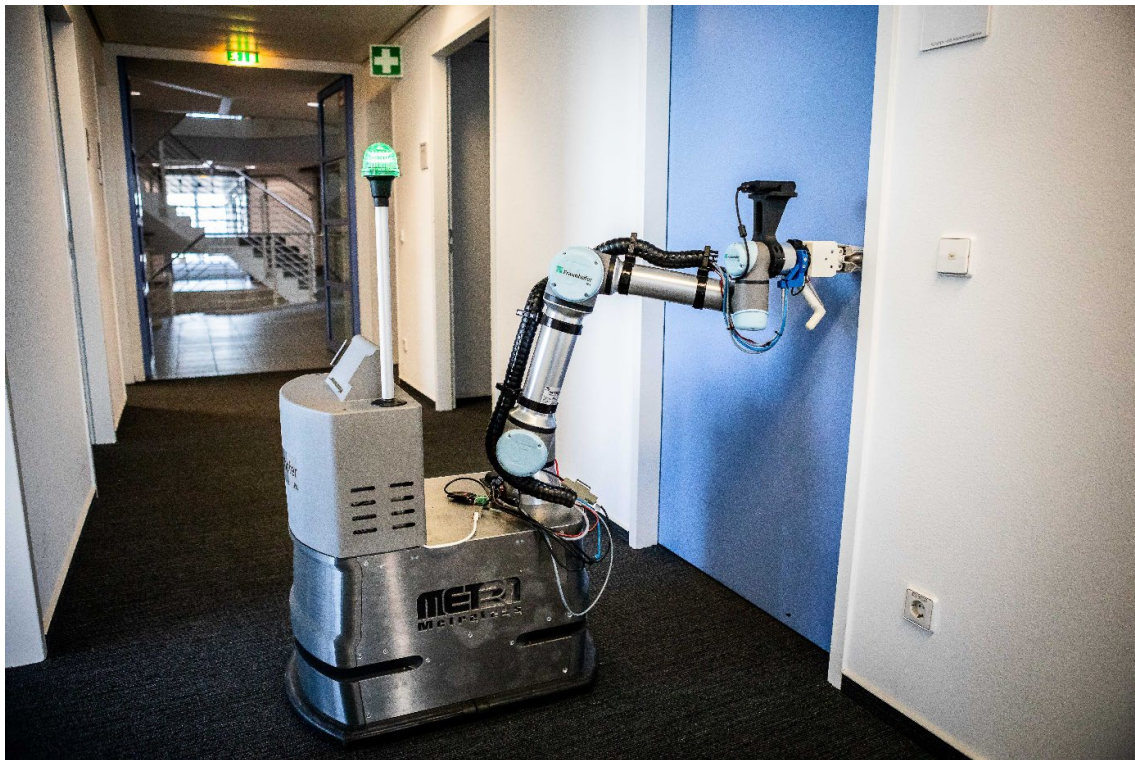
Figure 2.30: Using its cleaning brushes, DeKonBot 2 removes coarse dirt from door handles and comprehensively applies the disinfection fluid. Image credit: Fraunhofer IPA.
