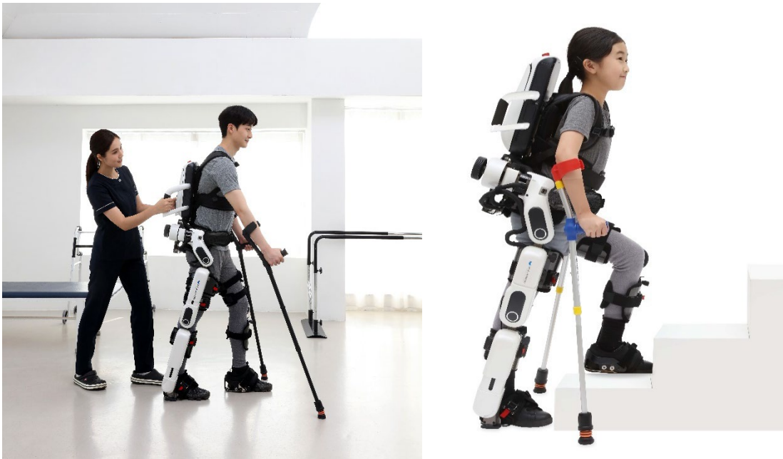
Figure 3.9: Angel Legs M is a gait-training robot for patients of any age with incomplete lower extremity paralysis. Image credit: Angel Robotics.
