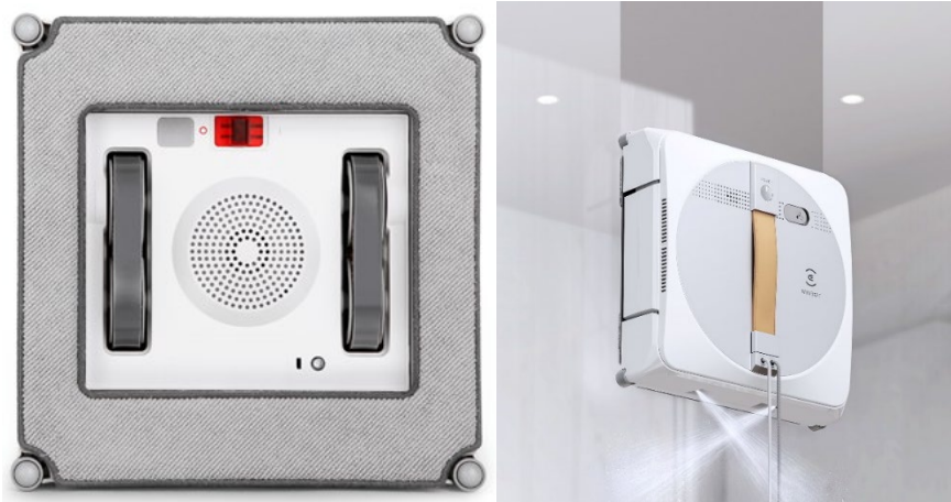
Figure 4.5: Winbot W1 Pro from Ecovacs Robotics cleans large windows automatically due to innovative cross-spray technology. Image credit: Ecovacs Robotics.
