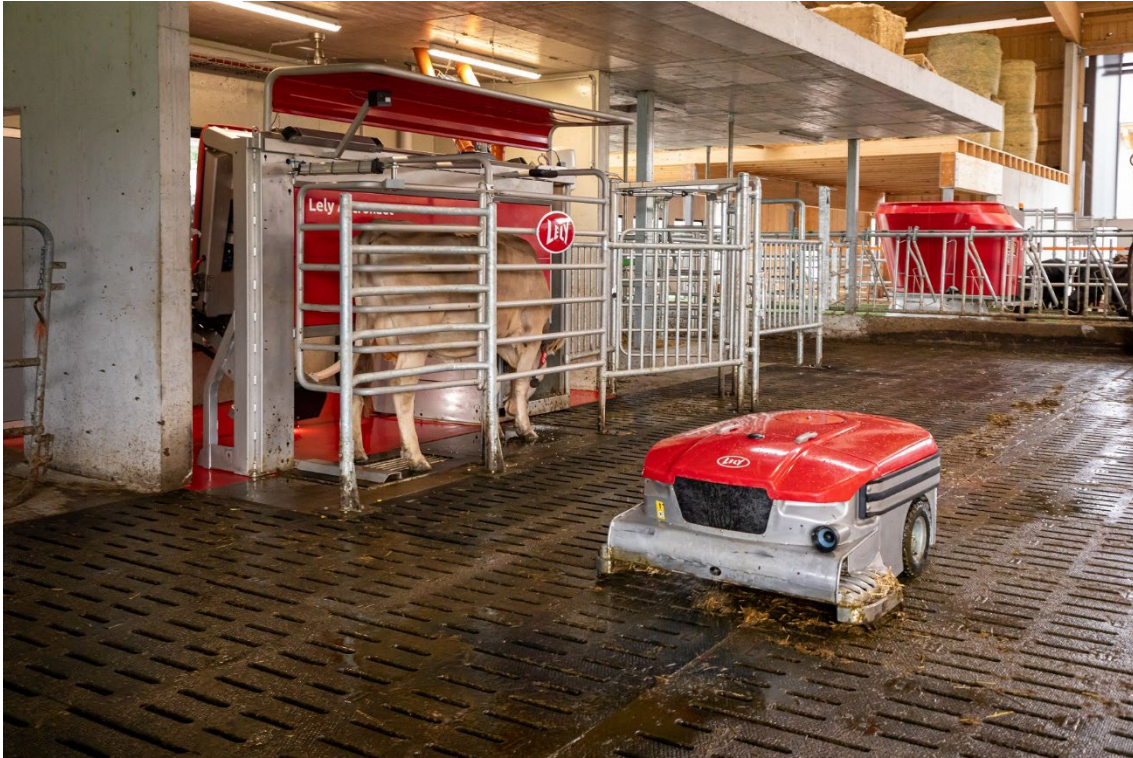
Figure 2.17: Several Lely barn robots: The Lely Astronaut Vector automatic feeding system, the Lely Collector barn cleaning robots, and the Lely Astronaut milking robot. Image credit: Lely International.
