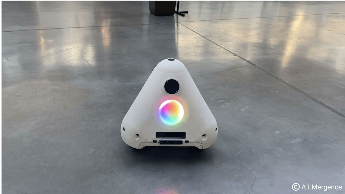
Figure 2.81: E4 is an autonomous patrolling robot that acts like a watchdog to secure premises and protect employees. Image credit: A.I.Mergence.
