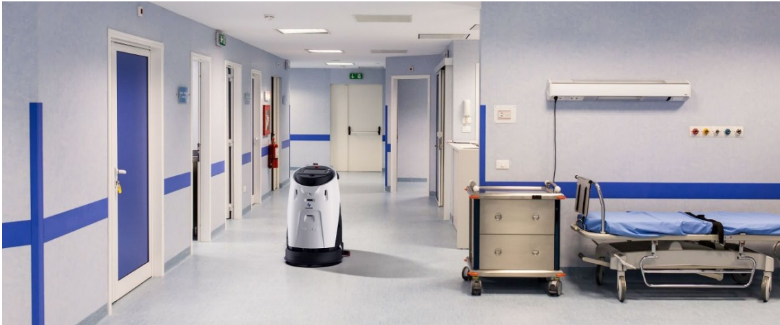
Figure 2.19: Gausium Scrubber in a health care facility. Image credit: Gausium Robotics.
