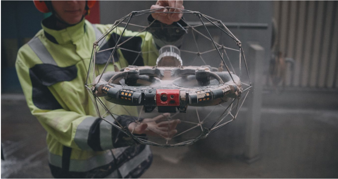
Figure 2.45: The Elios 3 created by Swiss drone company Flyability, designed for challenging, confined space inspections with a modular payload bay enabling a variety of applications across industries. Image credit: Flyability SA.
