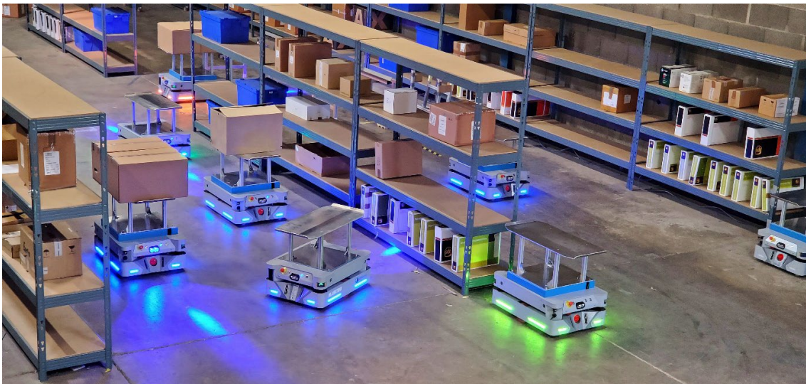
Figure 2.52: A fleet of Effibot-XS AMRs equipped with lift modules to enhance productivity. Image credit: Effidence.
