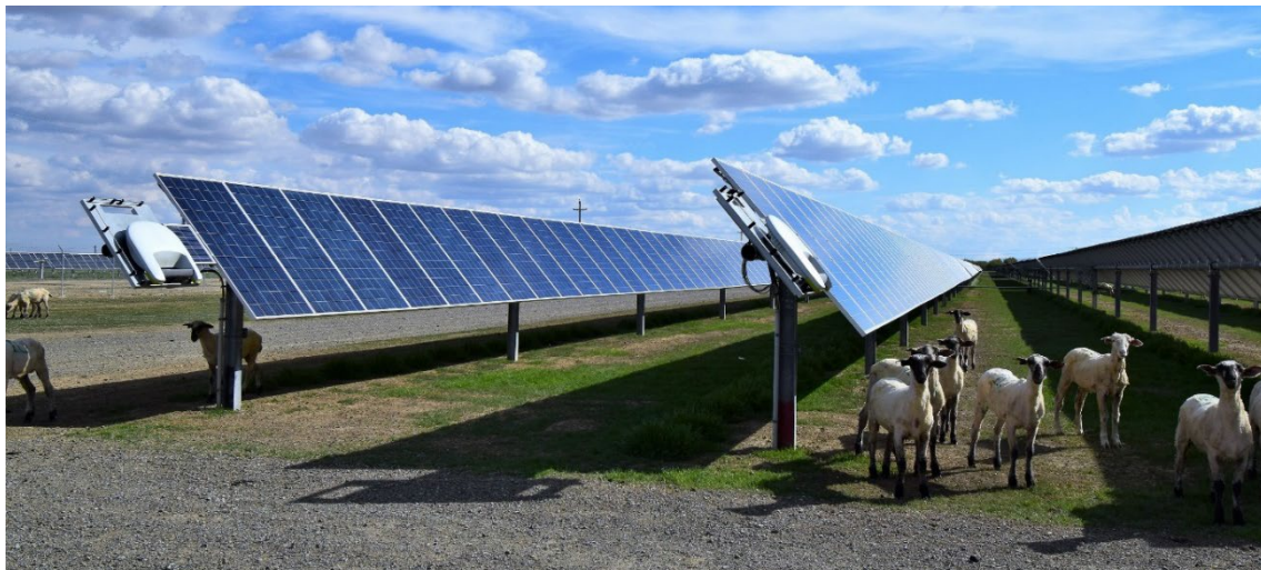
Figure 2.31: Ecoppia's fully autonomous, water-free solar panel cleaning robotic solution. Image credit: Ecoppia.
