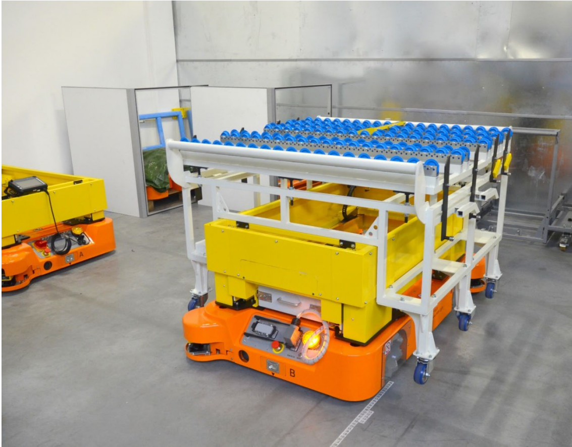
Figure 2.58: Mobot Flatrunner MW Light with gravity conveyor for the automotive industry. Image credit: Wobit.
