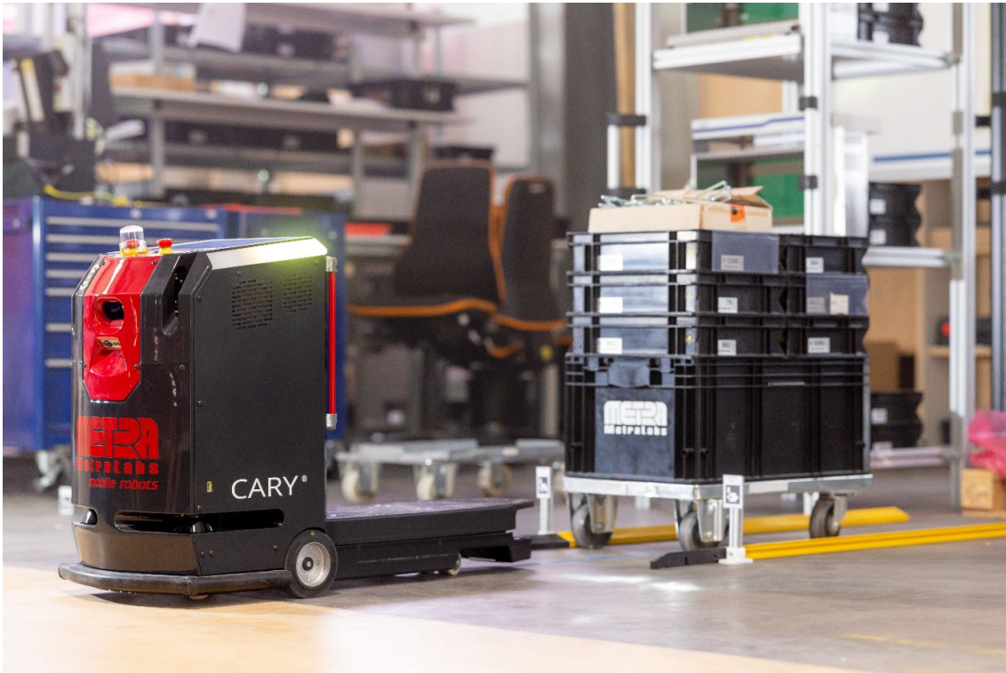
Figure 2.56: One more example of an AMR: Cary transports floor rollers autonomously through factories. Image credit: Metralabs.
