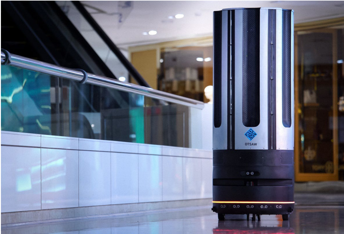
Figure 2.29: O-RX is a UV-C LED autonomous disinfecting robot with a disinfection rate of 99.999% at 2.5 meters. Image credit: Otsaw Digital.
