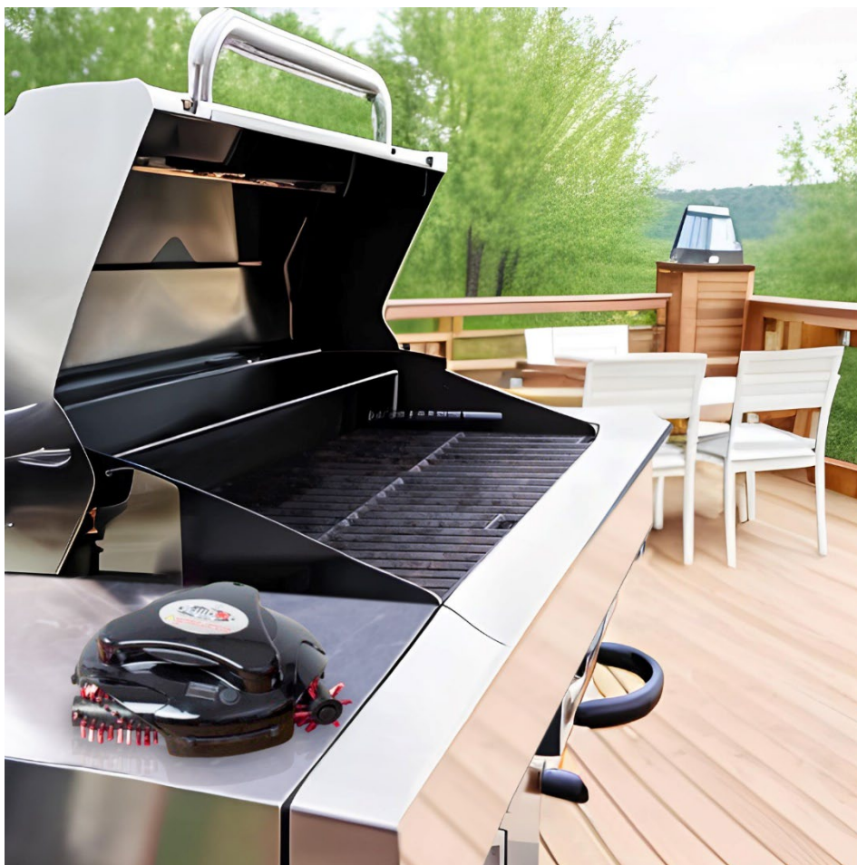
Figure 4.7: Grillbot is a small fully automated device with replaceable brushes and a rechargeable battery. Image credit: Grillbot.
