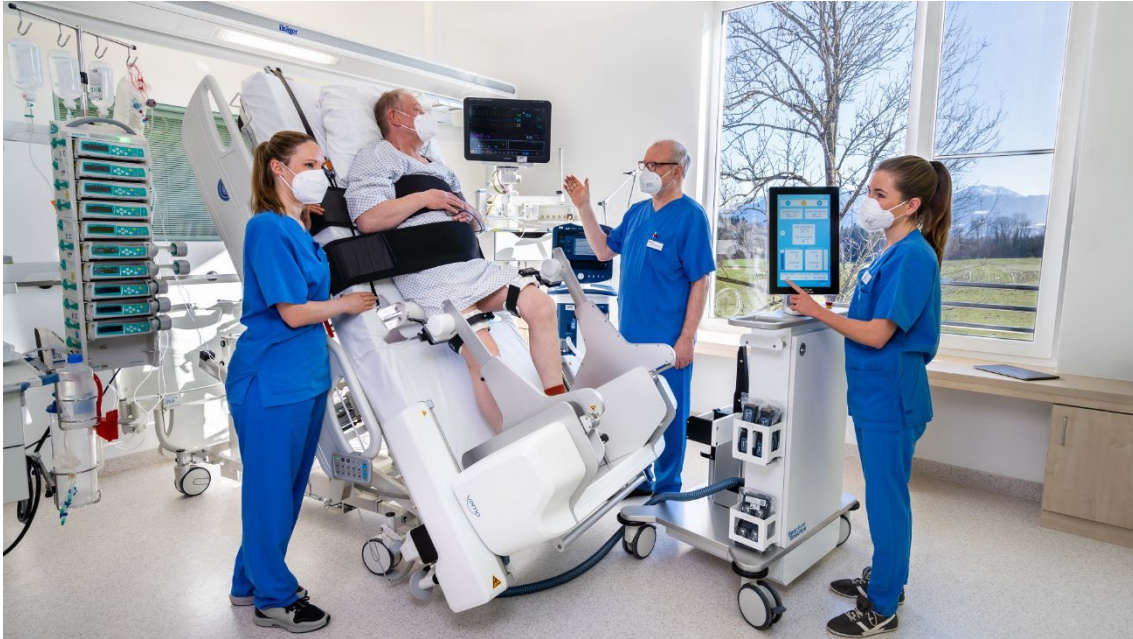
Figure 3.10: Reactive Robotics in the ICU: A robotics device equipped with artificial intelligence for the patient's individualized early mobilization therapy in the ICU. Image credit: Reactive Robotics.
