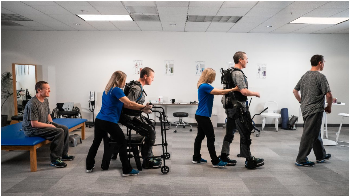
Figure 3.8: EksoNR™ – exoskeleton for the lower extremities for neurorehabilitation. Image credit: Ekso Bionics.
