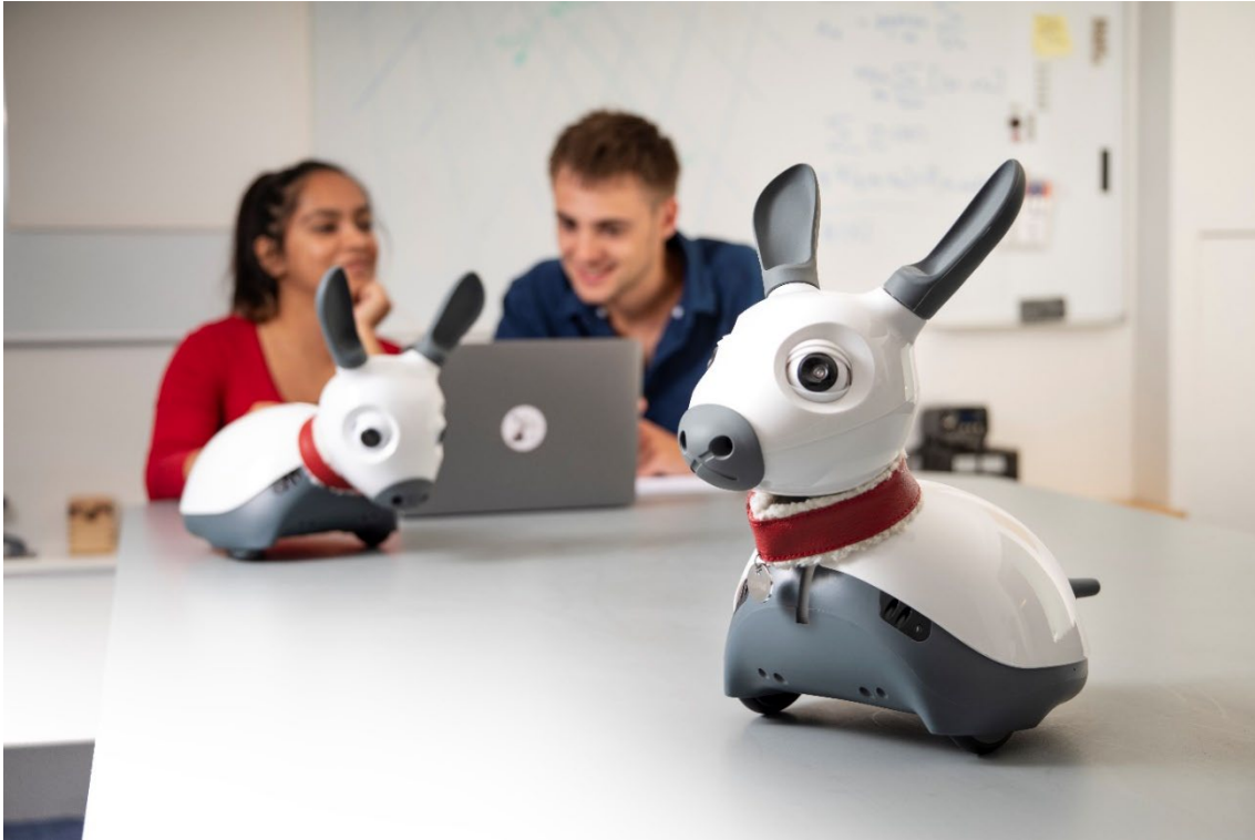
Figure 4.11: Miro is a fully programmable autonomous robot for researchers, educators, developers, and healthcare professionals. Image credit: Consequential Robotics.
