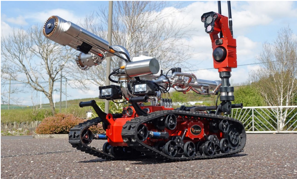
Figure 2.78: Avenger Fire provides firefighting crews with the capability to remotely manage a fire or other hazardous threats with a reduced risk to first responders. Image credit: ICP NewTech.
