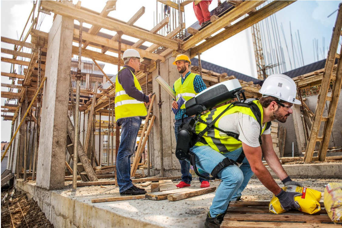
Figure 2.94: Exoback is useful for lifting heavy loads in professional works and jobs. Industry, construction, logistics are the main areas of interest for back support exoskeletons. Image credit: RB3D.
