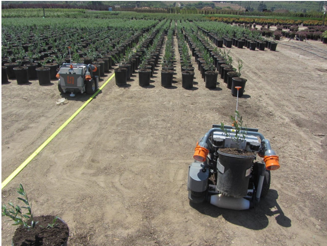
Figure 2.13: The HV-100 automates the most physically challenging task in ornamental horticulture production: The accurate placement of the plants in greenhouses or outdoors in any weather conditions. Image credit: Harvest Automation.
