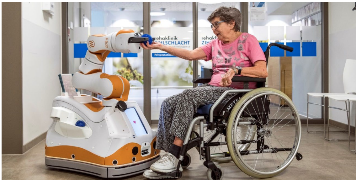
Figure 2.63: Lio is a service robot for various purposes in close contact with patients. Image credit: F&P Robotics.
