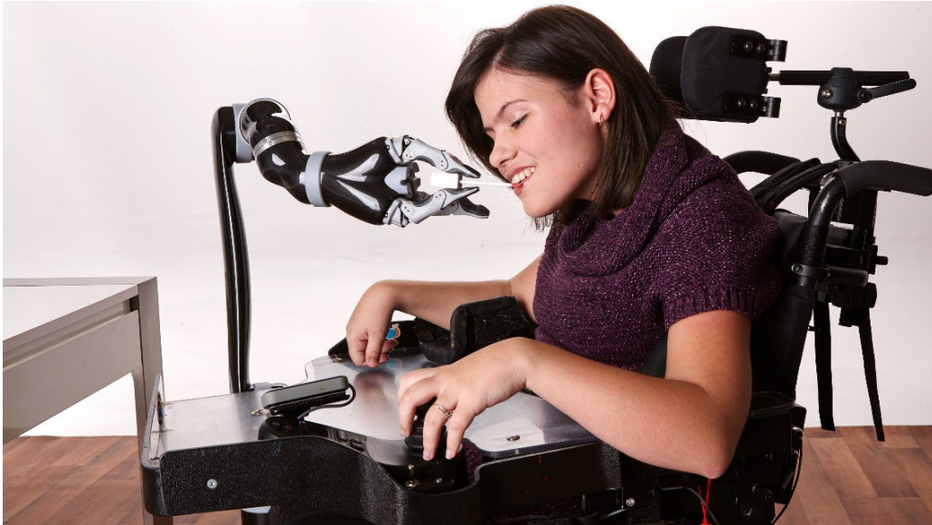
Figure 4.21: Woman with upper body limitations in a motorized wheelchair applying makeup using the Kinova® Jaco® assistive robotic arm. Image credit: Kinova.
