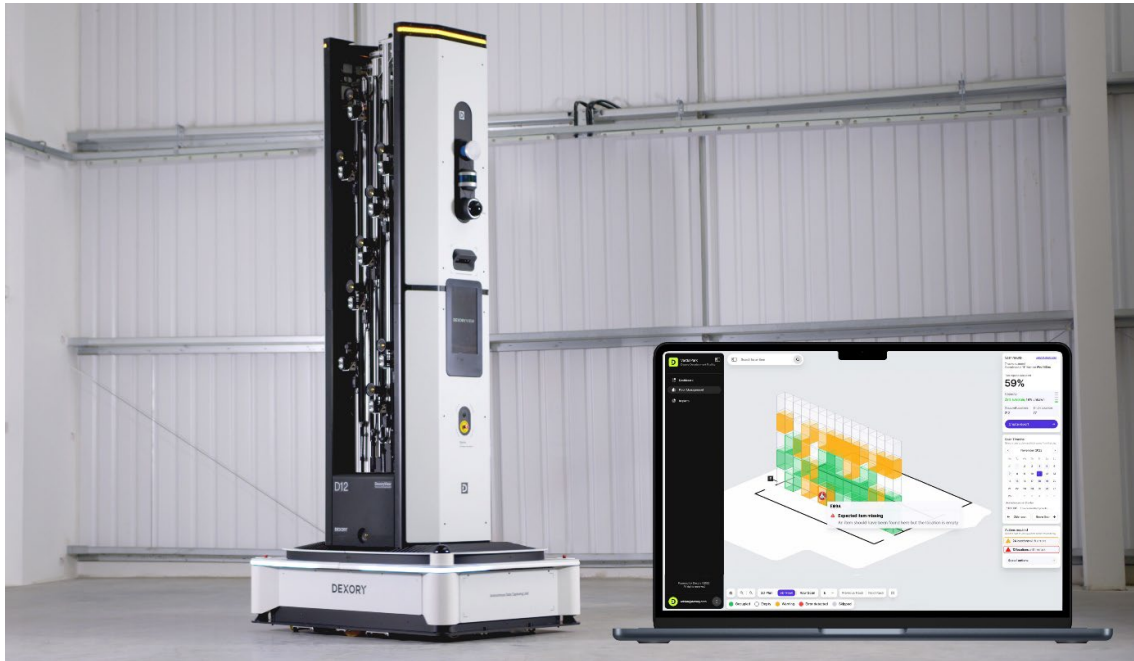
Figure 2.77: Dexoryview is a warehouse intelligence platform that helps logistics providers to maximize visibility of daily inventory operations using autonomous robots to gather accurate, real-time data and generate actionable insights. Image credit: Dexory.
