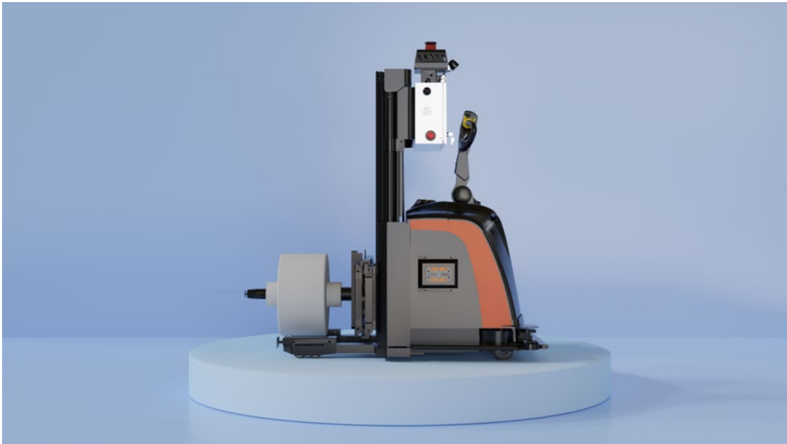
Figure 6.10: IPLUSMOBOT Omnidirectional Cantilever Forklift AMR. Image credit: IPLUSMOBOT.
