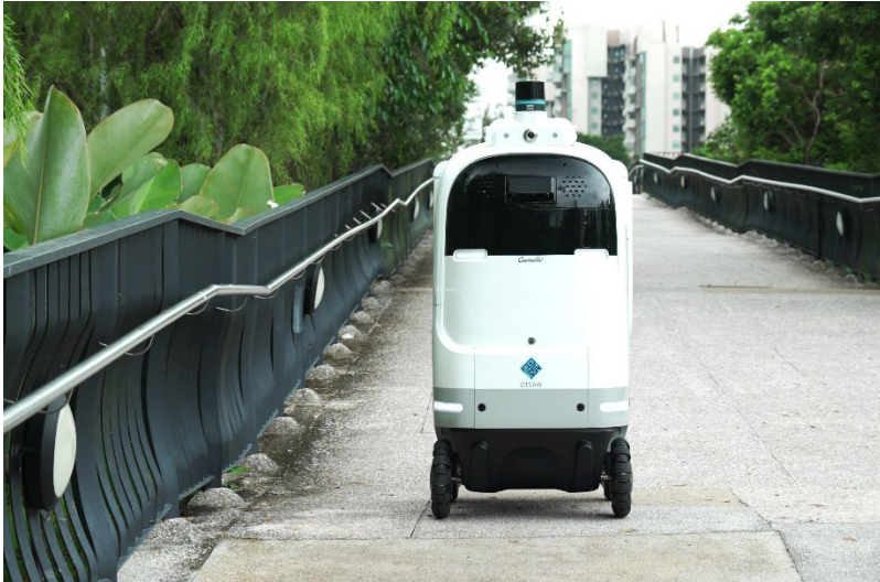
Figure 2.73: Otsaw Digital's autonomous last mile delivery robot. Image credit: Otsaw Digital.
