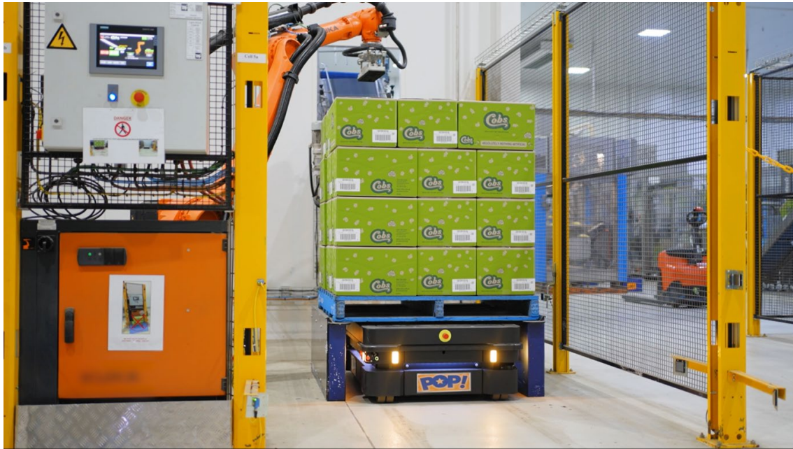
Figure 2.54: A fleet of MiR robots ensures a fully automated palletizing process at Kinrise Snackfoods. Image credit: MiR.
