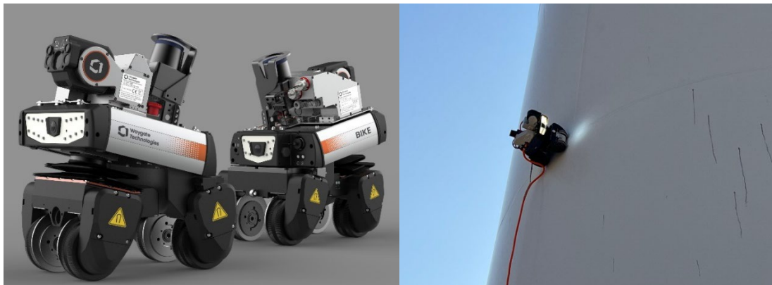
Figure 2.41: The Bike platform is a magnetic wheeled robot capable of inspecting power plant facilities and multiple applications in the oil and gas industry, such as vessel or pipe inspection. The locomotion concept allows the robot to climb obstacles like stairs and 90-degree corners (convex and concave). With integrated navigation cameras and 3D
