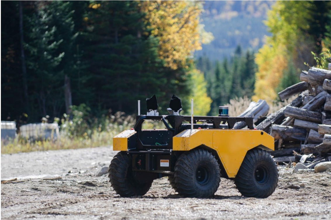
Figure 2.71: The Warthog unmanned ground vehicle from Clearpath Robotics can transport 272 kg. Image credit: Clearpath Robotics Inc.
