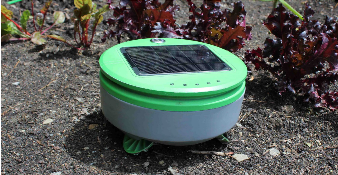
Figure 4.6: Tertill is a solar-powered, chemical-free, weather-proof robot that lives in domestic gardens. The robot measuring 21 centimeters in diameter eliminates the need for manual weeding. Image credit: Tertill Corporation.
