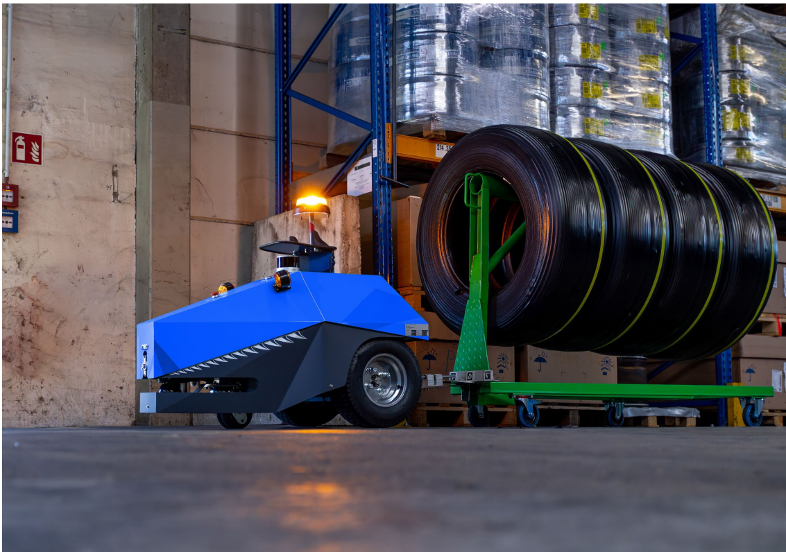
Figure 6.7: The Innok Robotics Induros AMR autonomously moves tyres between the production stations at the Innok customer Rigdon. Image credit: Innok Robotics.
