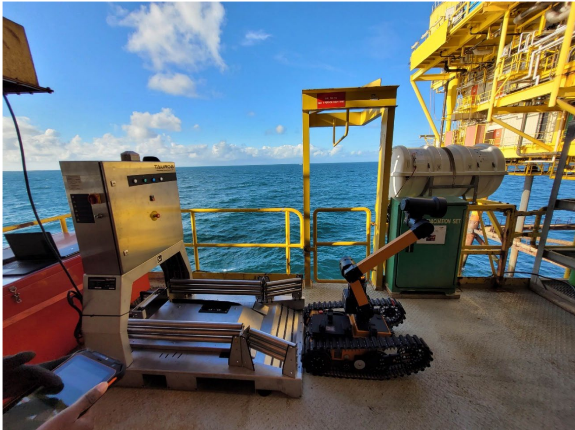
Figure 2.37: A Taurob inspector exiting its docking station to start an autonomous inspection mission on an offshore oil platform in ATEX mode. Image credit: Clemens Fröschl, Taurob.
