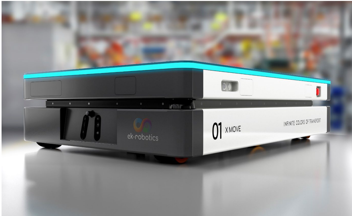
Figure 2.51: The X Move 2-in-1 transport platform can be equipped with a variety of load handling attachments. Three of the five models, with payloads from 150 kg to 1,900 kg, can be used either as AGVs or AMRs. The X Move transport robot supports the VDA 5050 interface and can be used in combination with other transport robotic systems. The image shows the X Move 1200. Image credit: Ek Robotics.
