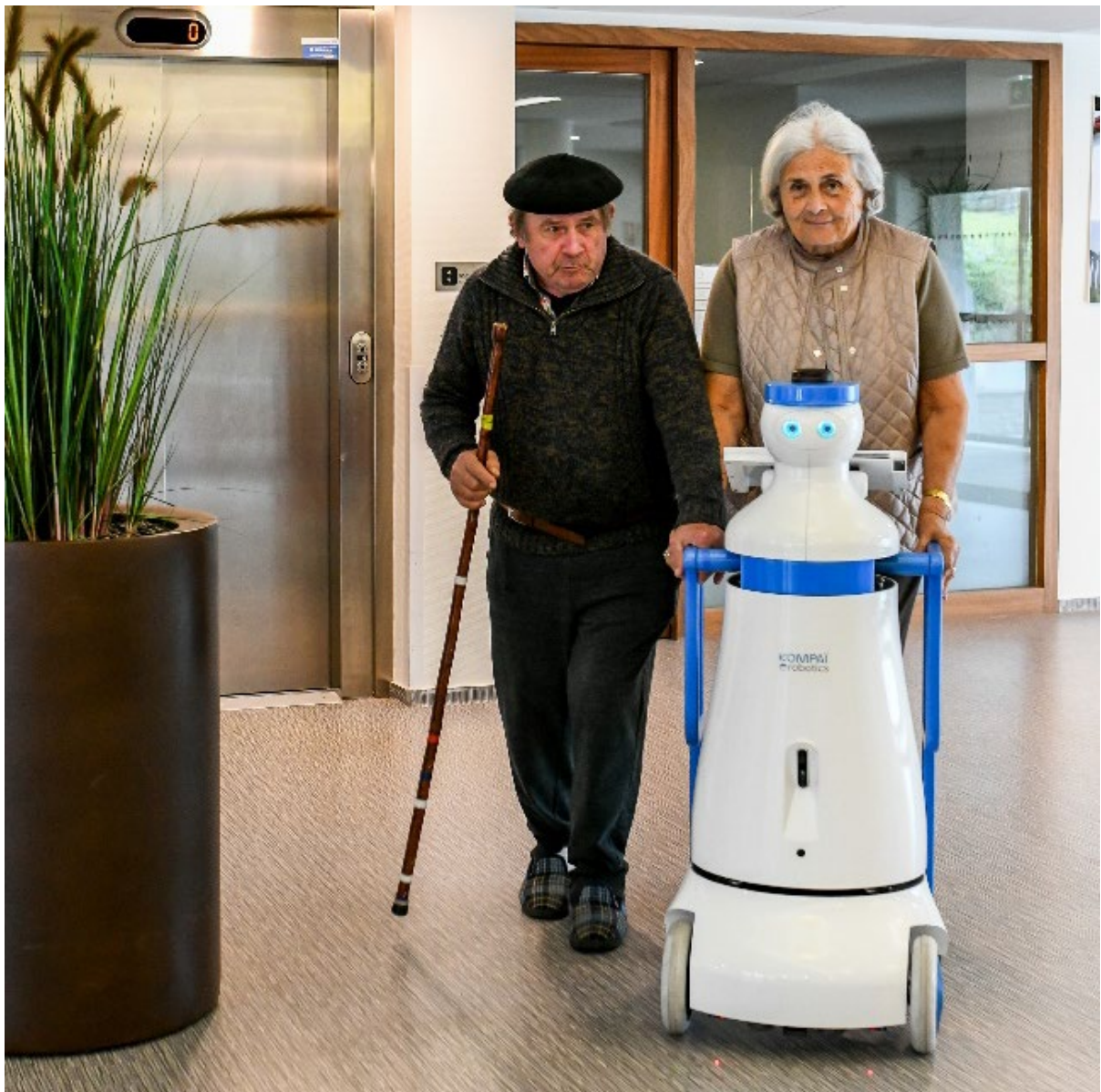
Figure 4.19: The robotic assistant Kompai offers functions like playing, cognitive exercises, maintaining social links, and can also be used as a walking aid. Image credit: Kompai Robotics.
