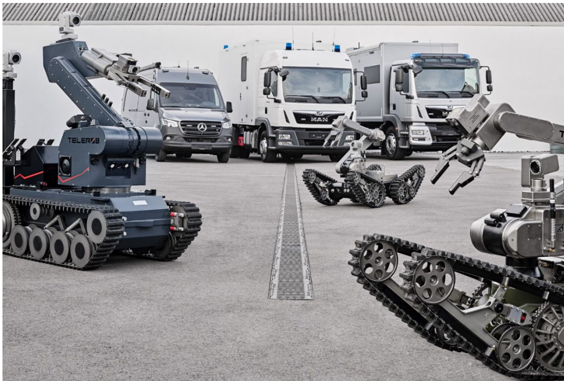
Figure 2.83: EOD (explosive ordnance) robot Telex EVO and EOD robot Teodor EVO with Telerob service vehicles. Image credit: Telerob Gesellschaft für Fernhantierungstechnik mbH.
