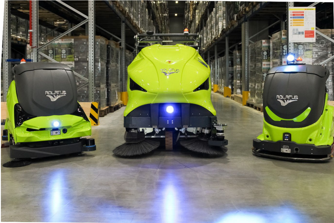
Figure 2.21: Depending on the application and the amount of dirt, Adlatus Robotics offers fully autonomous robot sweepers or scrubber-driers, all of which are equipped with a service station. Image credit: Adlatus Robotics GmbH.
