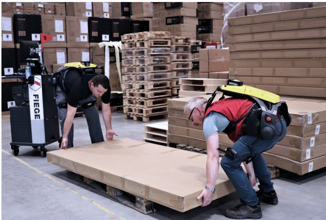
Figure 2.92: The Cray X power suit from German Bionic in operation at the Fiege Megacenter in Ibbenbüren, Germany, providing up to 30kg of active support per lifting movement Credit: German Bionic.
