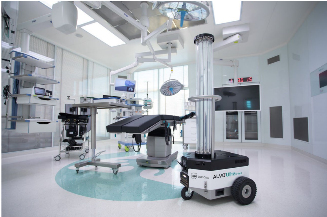
Figure 2.27: Alvo Ultra V-bot – disinfection in an operating room. Image credit: Wobit.
