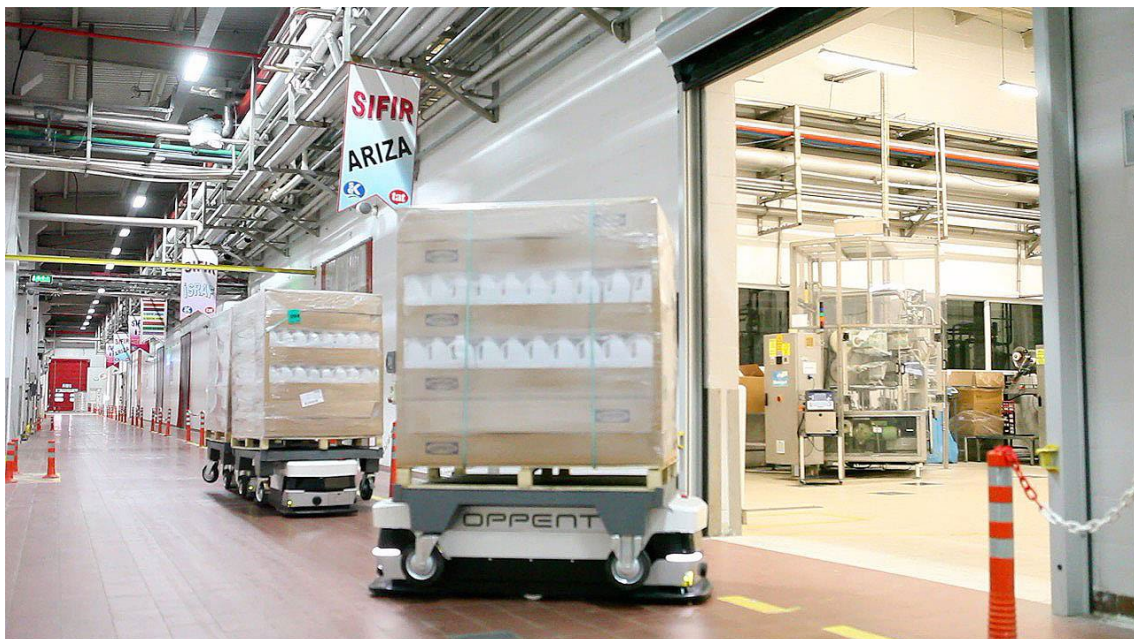
Figure 2.53: Evocart mobile robots from the Italian producer Oppent are used around the world to improve efficiency in logistics. Image credit: Oppent SPA.
