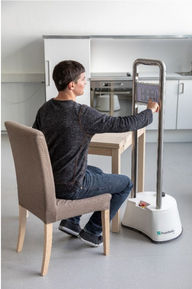
Figure 4.10: The mobile communication assistant Mobika supports telepresence, interaction, or reminder functions. Image credit: Fraunhofer IPA/Photo: Rainer Bez.
