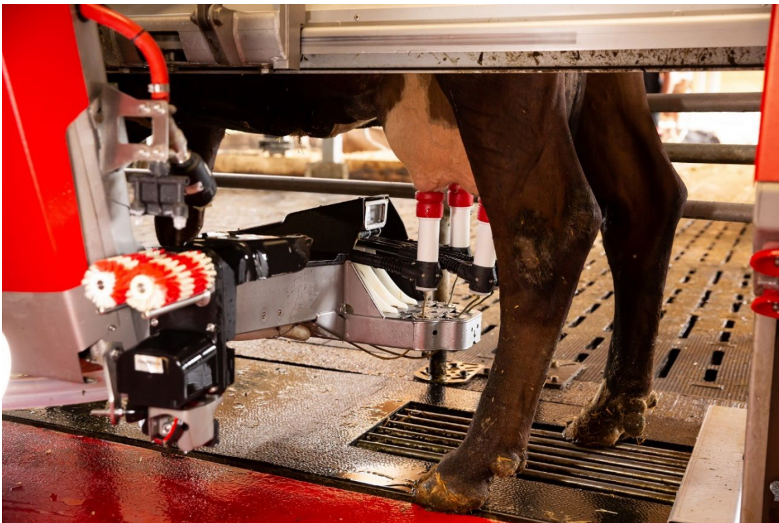
Figure 2.15: The Lely Astronaut A5 Automatic milking system, teat cups attached to the udder, shown from behind the cow. Image credit: Lely.
