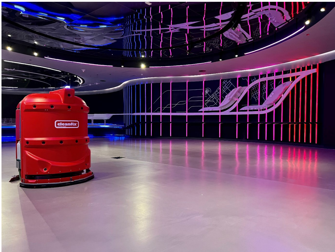
Figure 2.20: Cleaning robot RA660 Navi XL from Cleanfix – cleaning a tech center in Dubai. Image credit: Cleanfix Reinigungssysteme AG.
