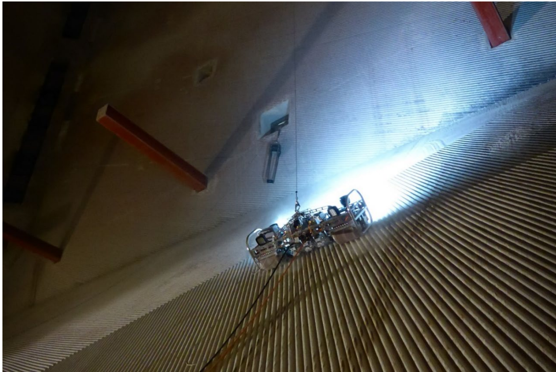
Figure 2.42: The service called BRIC (boiler robotic inspection & cleaning) will eliminate any physical risk to inspectors, provide precise data, and cut inspection costs for customers in sectors such as the chemical industry, paper manufacturing, or energy. Image credit: Waygate Technologies.
