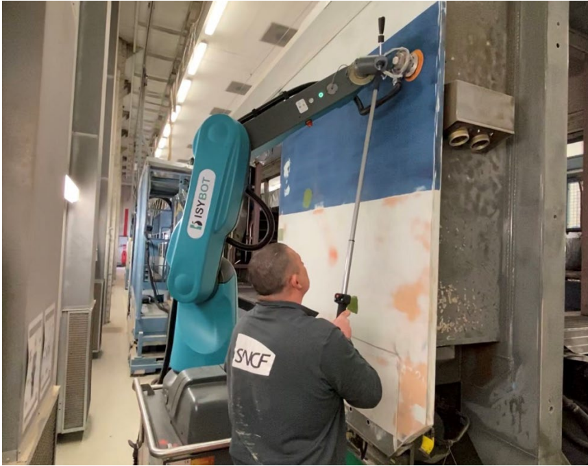
Figure 2.47: The Isybot collaborative system relieves the operator and increases the productivity in a variety of tasks, e.g. in the field of building construction. Here, a picture of the cobot SYB3 is shown in a configuration for a sanding application with the integrated vacuum system. This configuration of the cobot is currently used to sand walls in preparation for the final painting process. Image credit: Isybot.
