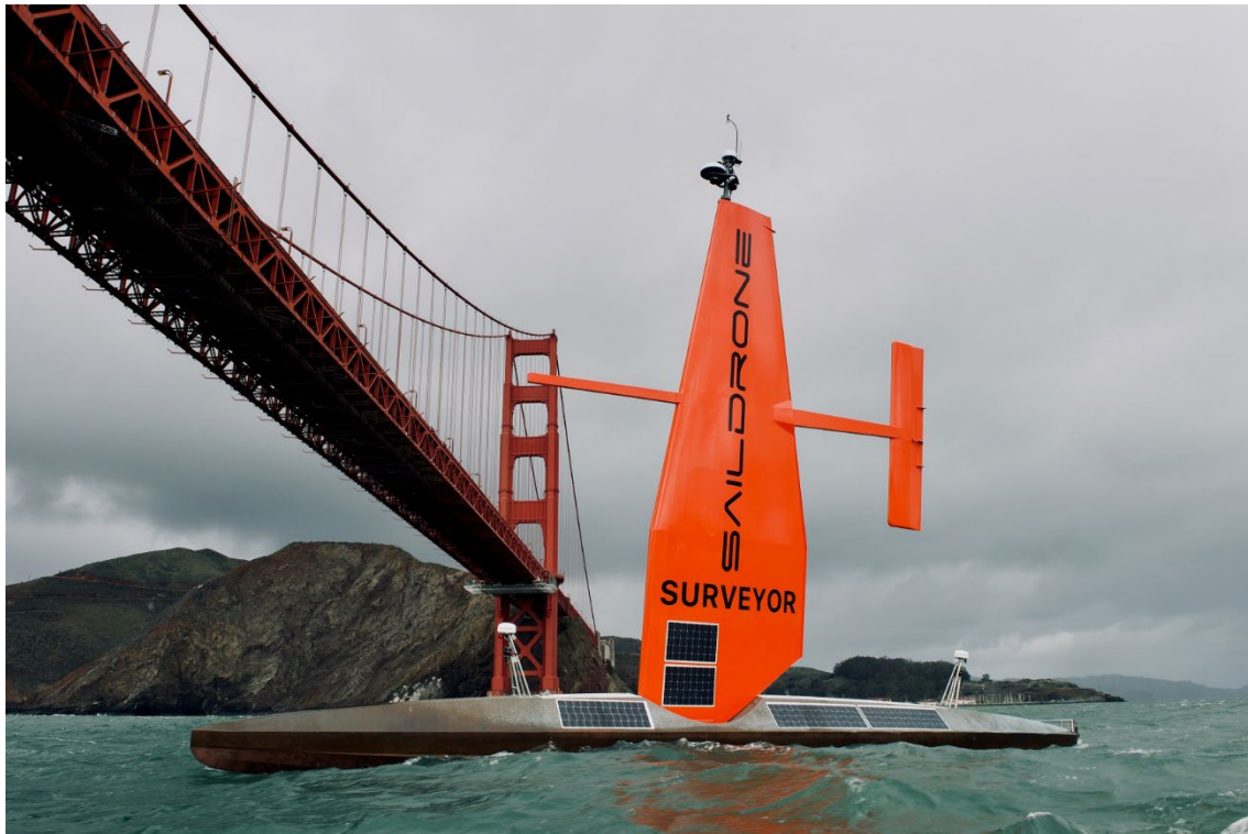
Figure 2.96: The 22-meter Saildrone Surveyor sails under the Golden Gate Bridge during sea trials in spring 2021. The Surveyor was first launched in January 2021 and is specially equipped with a suite of multi-beam sonars for deep-water ocean mapping, as well as fisheries sonars and an acoustic Doppler current profiler to measure ocean currents. Image credit: Saildrone.
